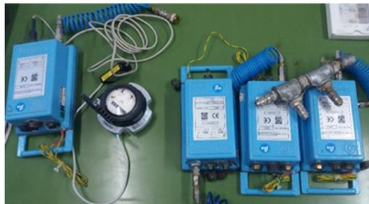
*Figure 5.2. Data loggers used for pressure measurements.*
