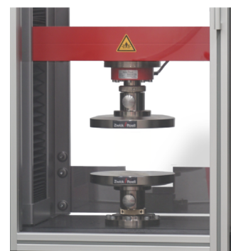
Figure 28. Compression test on springs. From ZwickRoell, n.d, https://www.zwickroell.com/products/static-materials-testing-machines/universal-testing-machines-for-static-applications/proline/ , Copyright by ZwickRoell
