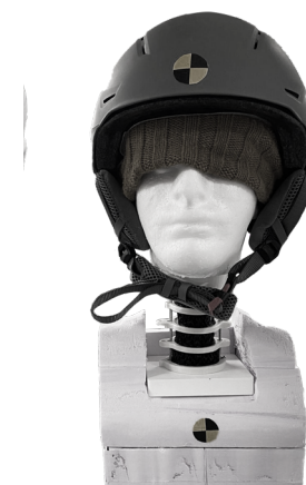
Figure 26. Test Dummy's Necks a) Neck Mounting Platform Assembly. From THOR-50M 472-0000 THOR-50 th Percentile Male Dummy User Manual 472-9900 [Rev. F] , 2018, by Humanetics Innovative Solutions, ©2018 Humanetics Innovative Solutions Inc. b) Neck made for test set-up, Own Photograph
