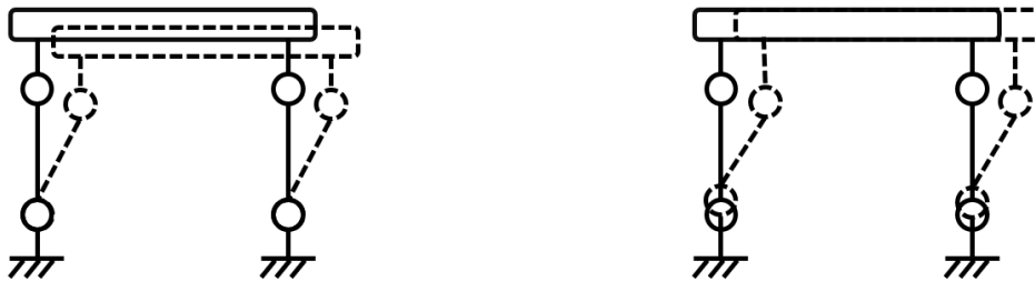
Figure 3.7: Visualization of the compensation within the mechanism. On the left without compensation. On the right with compensation (the rotation points change in vertical position during deformation).
