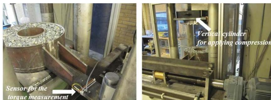
Figure 5: Shear-Compression Machine
