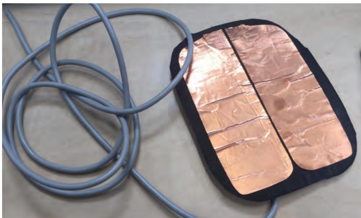
Figure 6.5: Reusable patient plate including a safety monitoring system.
