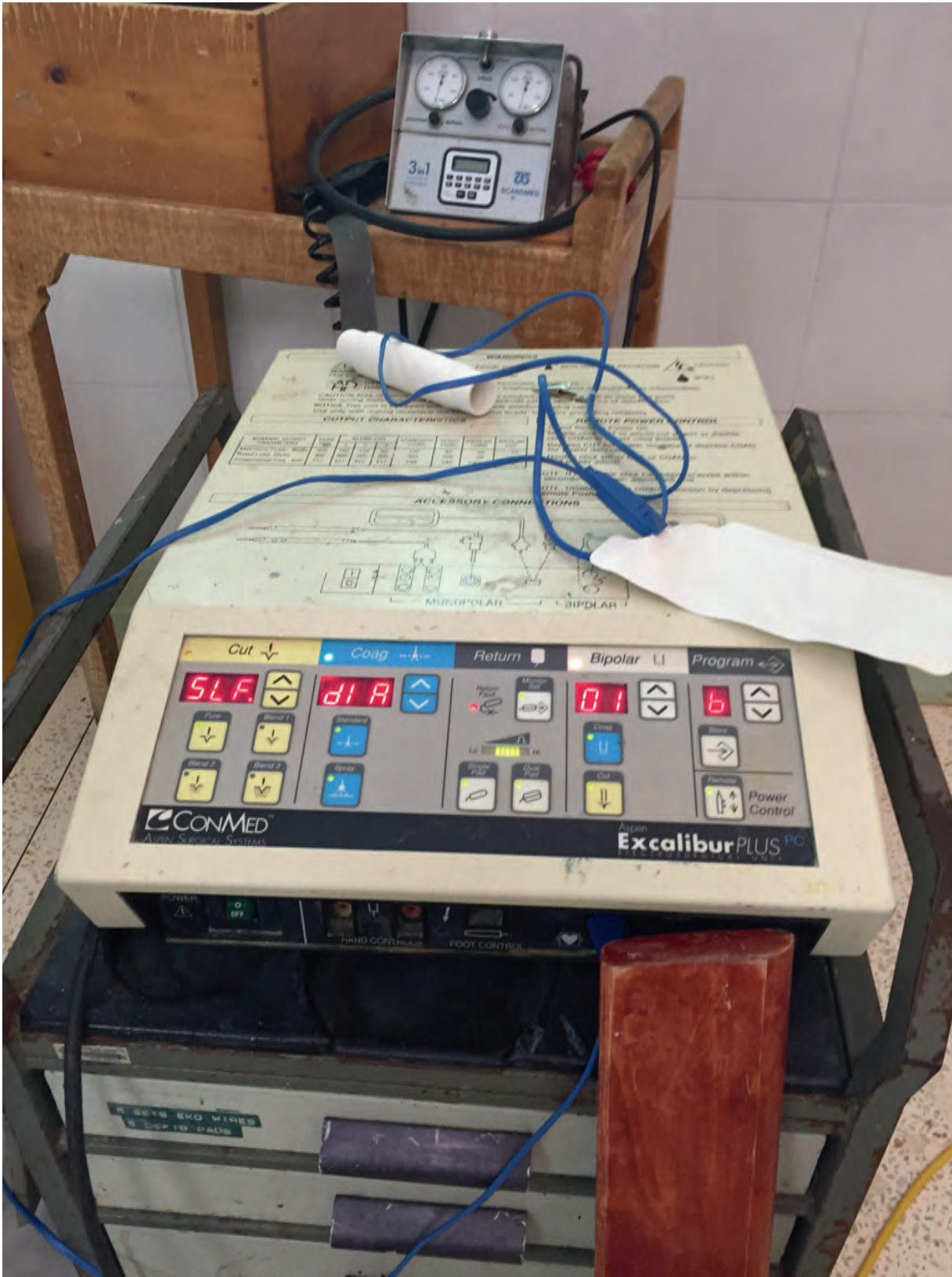
Electrosurgical unit in a large hospital in Kenya with a patient plate sticker.
