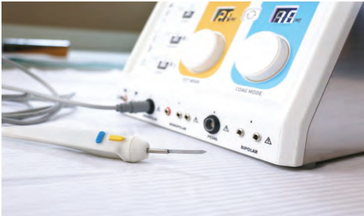
Figure 6.4: Non-functional concept prototypes of the ESU and monopolar handheld that were used for further evaluation of the designs. * A redel connector was used for this prototype because it was easily accessible during the manufacturing of this prototype, the 3x 4mm banana plug will be used for future prototypes.
