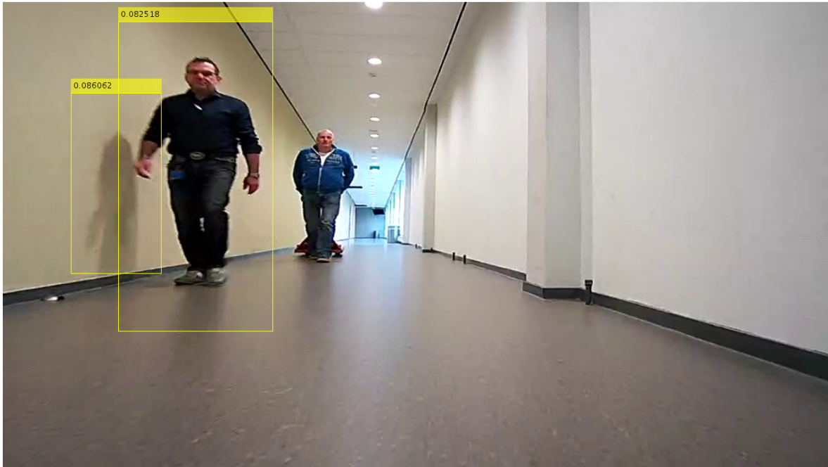
Figure 5-18: More results using the sliding window HOG-SVM classifier.
