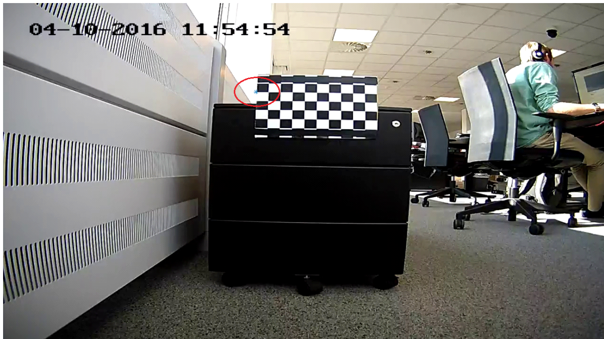
Figure 3-3: The calibration setup with one laser scan point projected on the checkerboard.
