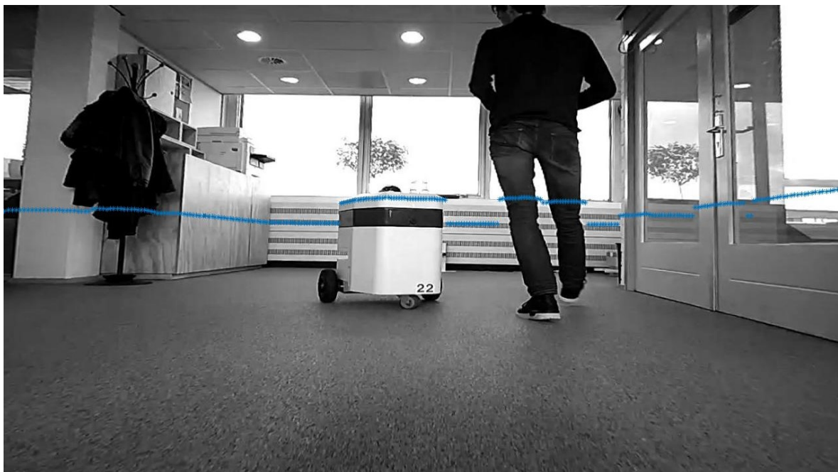
Figure 3-5: A projected laserscan after data synchronisation and undistortion.
