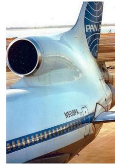
Figure 8.9: Lockheed L1011 S duct<sup>8</sup>
