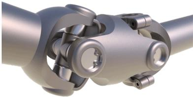
Figure 8.6: Double Cardan joint<sup>5</sup>
