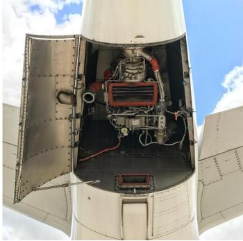
Figure 8.8: A320neo APU inlet<sup>7</sup>
