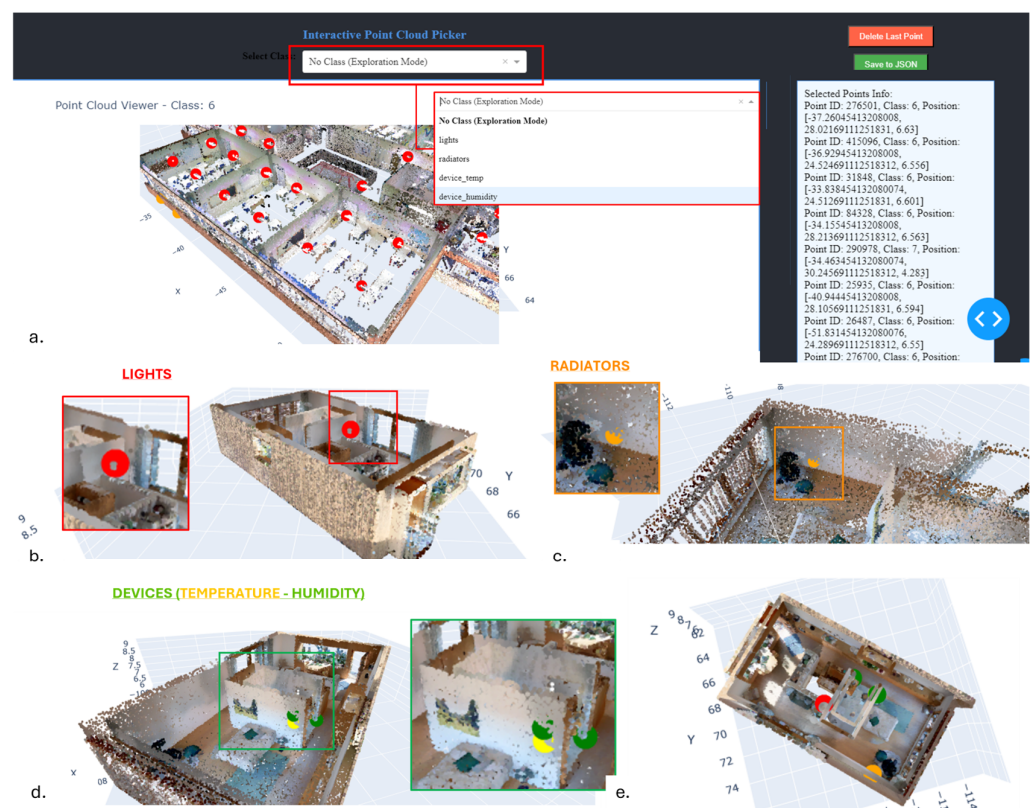
Figure 6. Results of the developed tool for manual energy-element detection and classification: (a) interface and lights, (b) lights, (c) radiators, (d) devices/sensors, (e) top view after detection.
