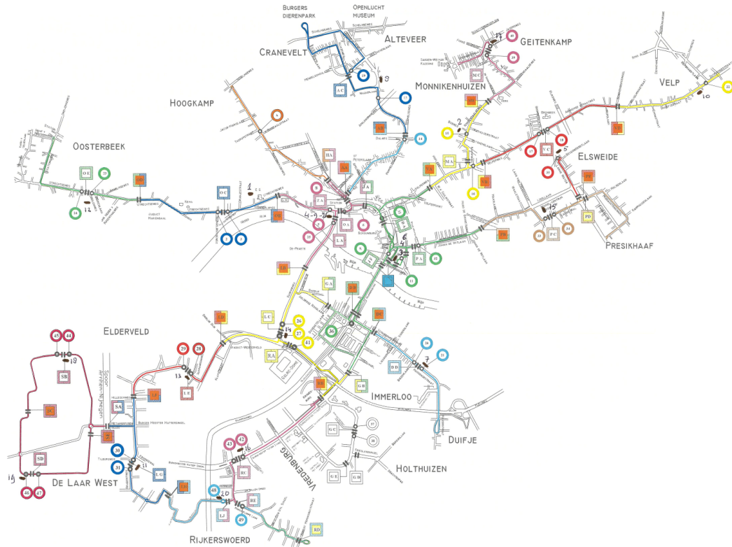
Figure 3.1: Map of the Arnhem trolley-grid showing sections and substations.
