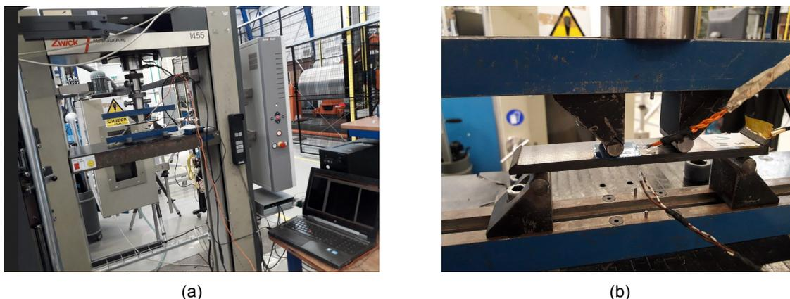
Figure 3.9: Low-frequency bending. (a) gives the general arrangement. (b) shows the real-life placement of the specimen.
