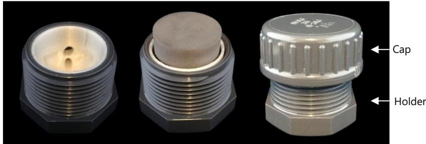
**Fig. 33** PVC parts (cap and holder) with mould and sample.
