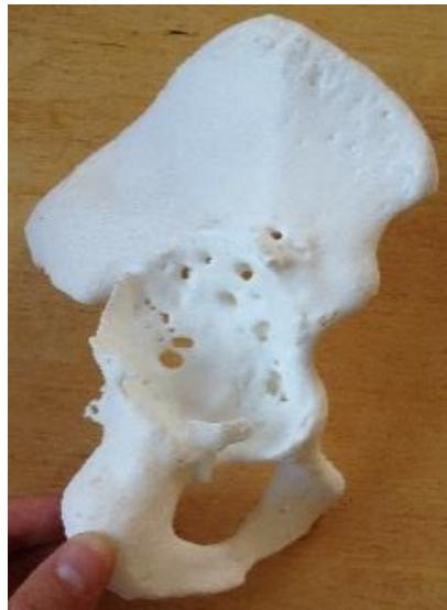
**Fig. 2** Acetabular model printed with FDM printer.
