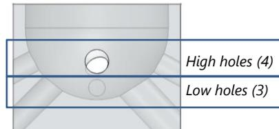
**Fig. 21** Relatively high and low positions of the holes in the mould.
