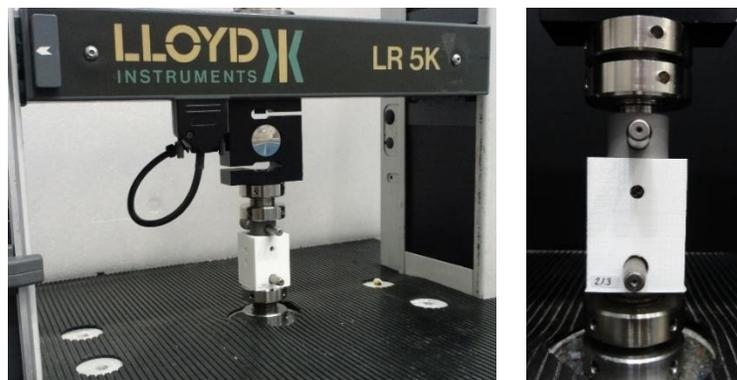
**Fig. 19** Set-up before the start of pull-out test.
