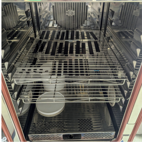
Figure 4.8: Weiss LF7m45 climate chamber used for controlled hygrothermal aging of specimens.
