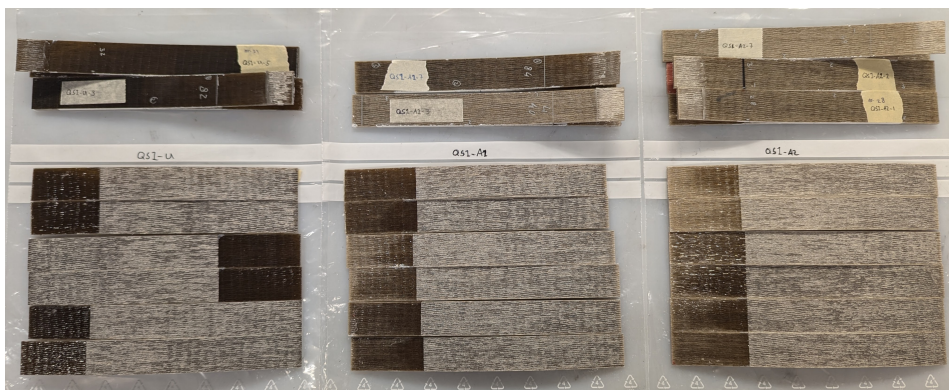
Figure 5.11: Mode I fracture surfaces, unaged (left), 1-cycle (middle), 2-cycle (right).
