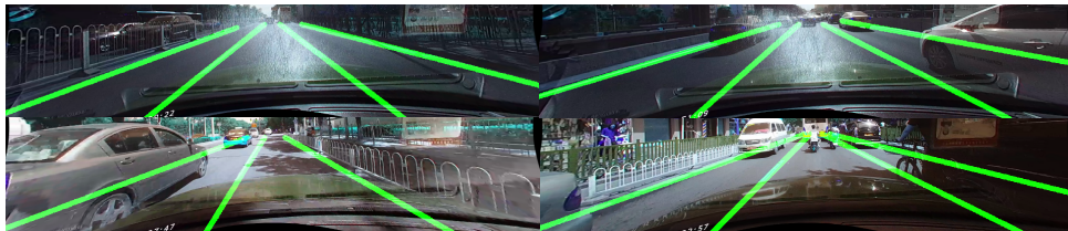
Figure 1.4: Traffic lane detection. The ground truth is annotated in green. Illumination variation and traffic flows are challenging for lane detection.
