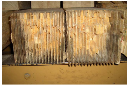
Figure 4.8: Damaged glue laminated box girder [82]
