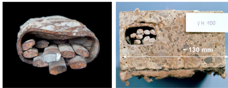
Figure 4.3: Poor workmanship of pre-stressed tendons [31]
