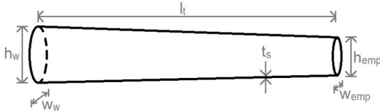
Figure 8.9: Configuration of the tail beam
