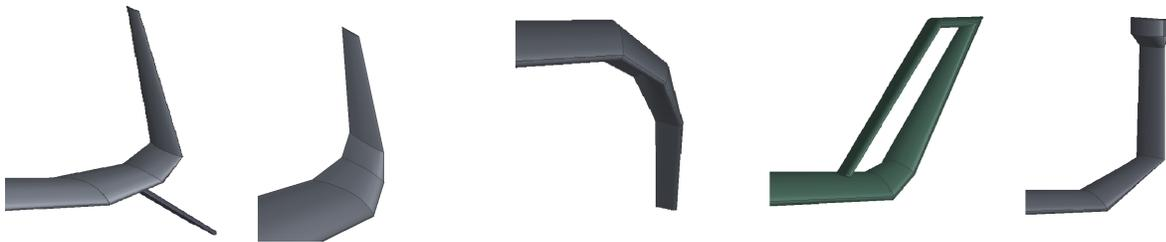
Figure 5.10: The four investigated winglet designs are shown, from left to right: the double winglet, integrated winglet, dropped winglet, spiroid winglet and the final design.
