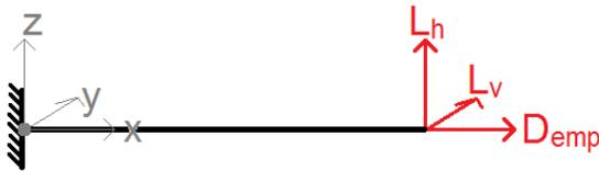
Figure 8.11: Free body diagram of the tail beam during nominal flight
