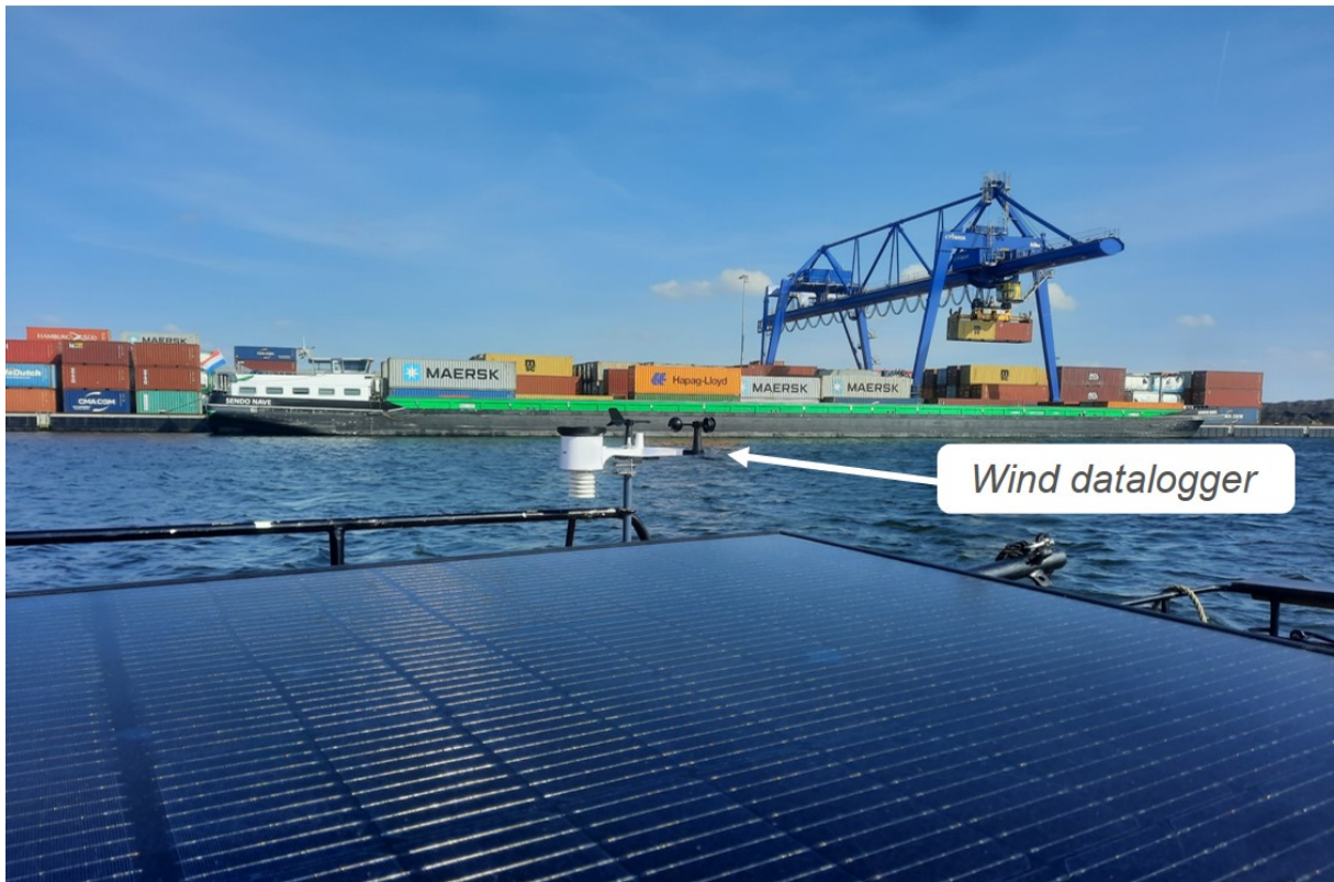
Figure 3.37: Wind data logger with a container vessel in the background
