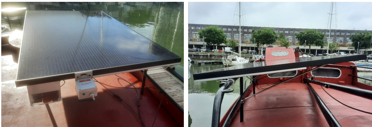
Figure 3.31: Harmonie's panel tilt: zero degrees(left) and eight degrees to port side(right)
