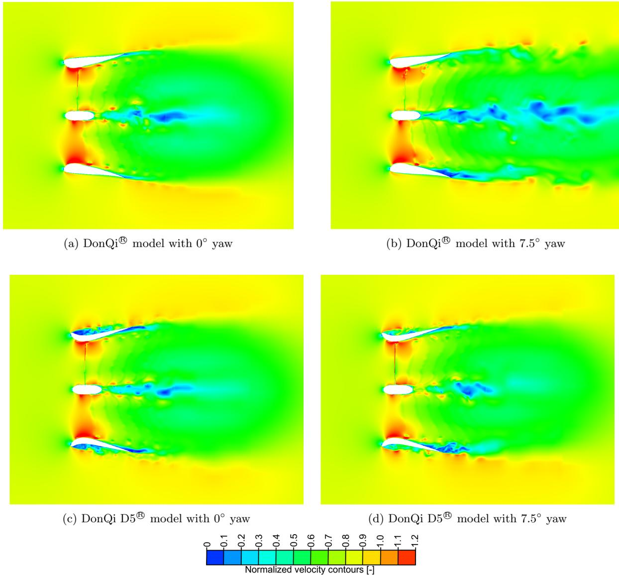
Figure 3: Velocity contours colored with normalized streamwise velocity.
