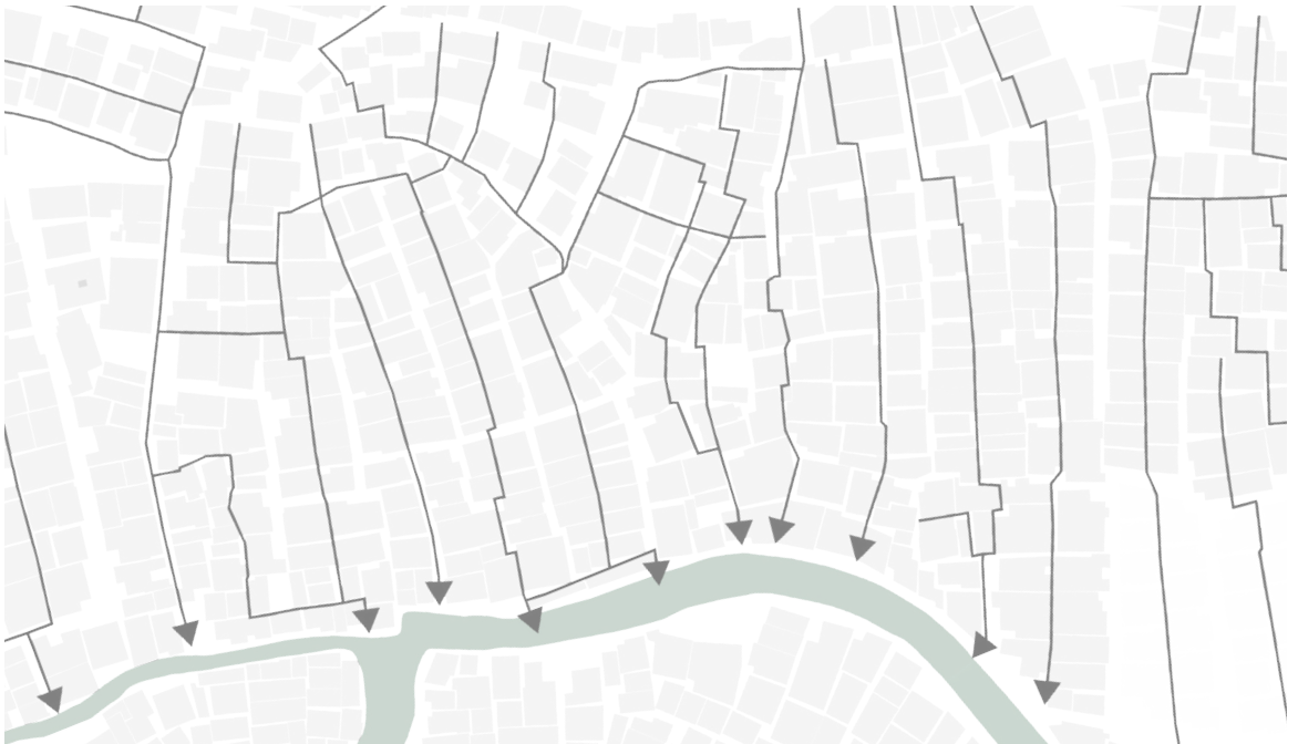
Img 10.6 - Existing sewage structure (Source: Authors own)
