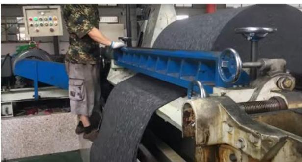
Figure 12: Peeling process of a cold moulded rubber cylinder
