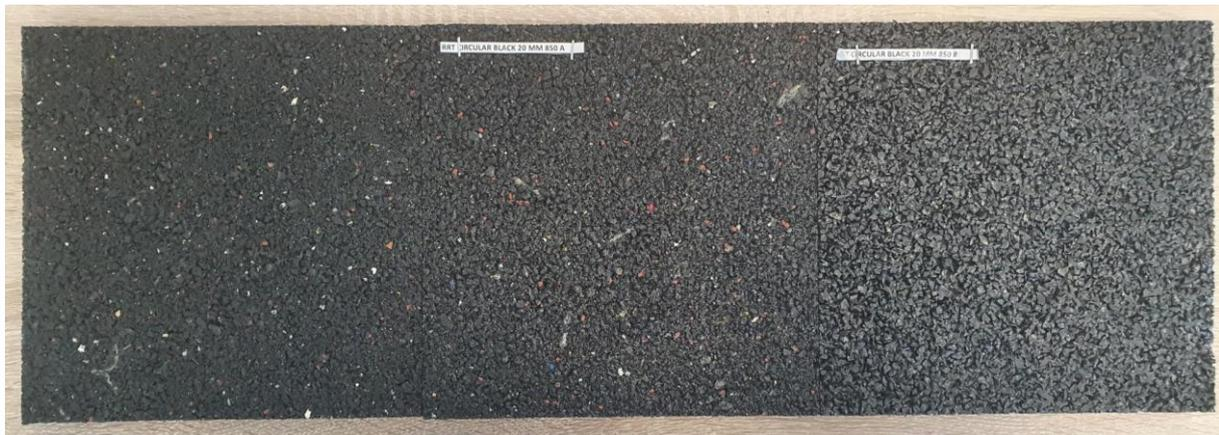
Figure 37: Test 2 – Used connect tiles recycled and made into standard tile – bottom view (from left to right A, B, C)
