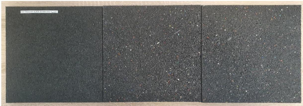
Figure 36: Test 2 – Used connect tiles recycled and made into standard tile – top view (from left to right A, B, C)
