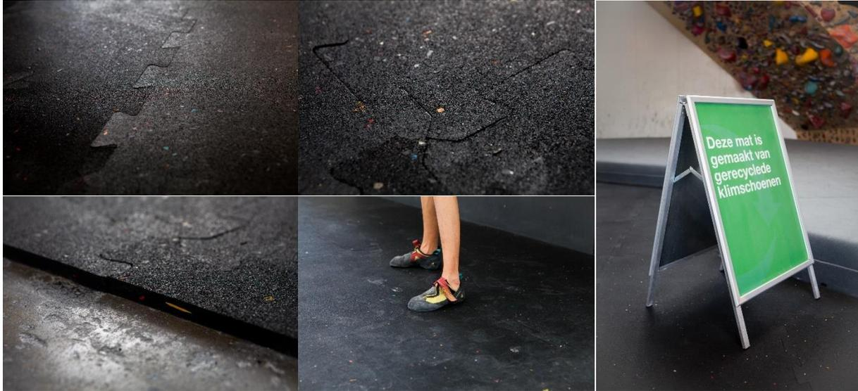
Figure 34: Climbing shoe tiles, 10% climbing shoe with 90% car tyre granulate
