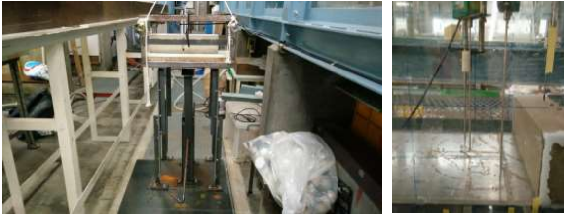
Figure 3. Experimental Apparatus. Left: Weight system to release the gate. Right: wave gauge and velocity meters
