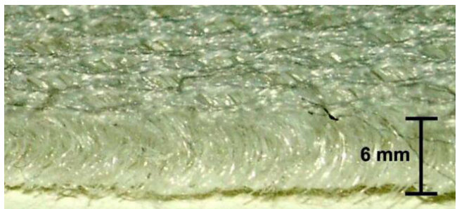
Figure 6.5 3D knitted spacer in Müller Textil, Germany (Meyer et al., 2010)
