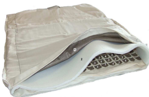
Figure 2.2.8 Textile sensor with 240 elements used for sitting posture measurement. 1: common electrode, 2: spacer, 3: sensing electrodes, and 4: electrodes switched to ground. (Meyer et al., 2010)
