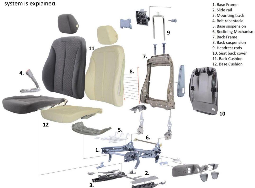
Figure 4.1 Exploded view of a typical modern car seat, BMW 3 Series 328i (A2mac1 2014) (Jakob Steinwall, 2014)
