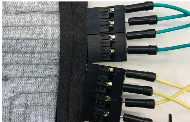
Figure 5.21 Crimping connection with the conductive yarns stitched in a wider gap.
