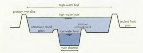
Schematic cross-section of the high-water bed from an embanked river.
