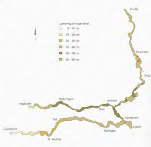
Reduction of the design flood water levels when the embanked flood plain is lowered by 1.0 m.
