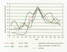
Comparison of the flood waves on the Rhine in 1926, 1993 and 1995.
