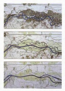
In 1800, Johann Gottfried Tulla started with the standardisation (fixation of the main river bed) of the Upper Rhine. The maps present the Upper Rhine at Breisach before and after Tulla's correction around 1828 and after the last canalisation in 1963. As a result of canalisations less space was left for the river Rhine.
