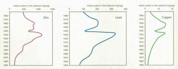
Sediment deposited in a pond within the embanked Waal flood plain, reflects the history of the metal pollution of the Rhine.
