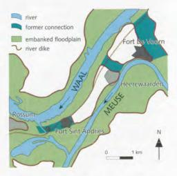
Former connections between the Waal and the Meuse. When the Waal discharge was high, water spilled from the Waal into the Meuse.
