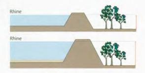
Dike raising will finally lead to a larger inundation depth, and therefore more damage, when a dike should burst.
