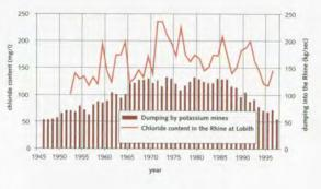
Salt dumping and chloride contents in the river Rhine.
