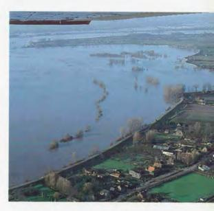
High discharge through the river Waal. The polders here are like bathtubs behind the river dikes. A polder will be flooded within a day in case a river dike breaches. The inundation depth, then, will be several meters.
