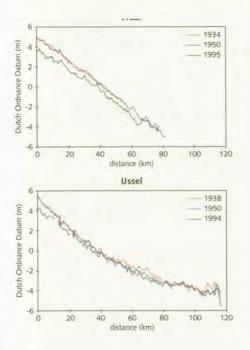
Level of the bed of the main channels of the rivers Waal, IJssel and Nederrijn-Lek in this century.
