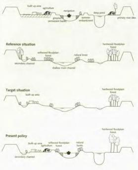
Cross section of the high-water bed in the present situation, according to the reference situation, the target situation, and by continuation of the present policy.
