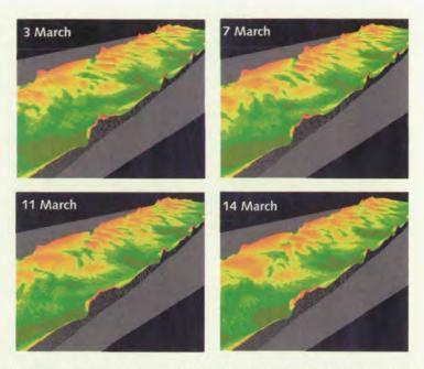
Migration of river dunes on the main channel bed of the river Waal during the 1997 flood. The river bed topography of a 1 kilometre reach is shown for 4 successive time steps between the 3rd and 14th of March 1997. Dunes up to 2 metres high have been observed. The river flows from right (behind) to left (front).
