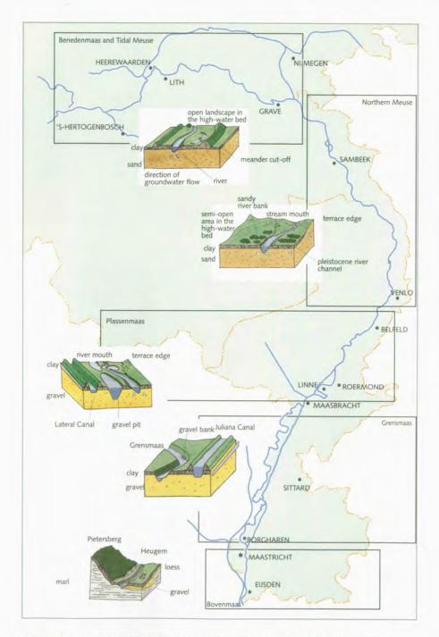
Meuse sections: schematic representation of cross-sections and composition of the sub-soil per section.
