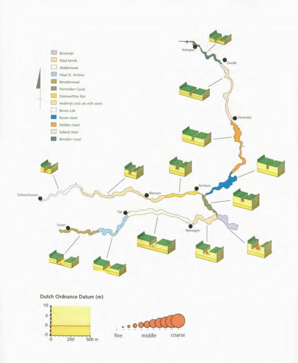
Rhine branches with cross-sections and grain size of the bed material per section.
