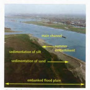
During flood periods, sand is deposited by the river on its natural levees. Deposition of silt and clay occurs behind the summer embankment.
