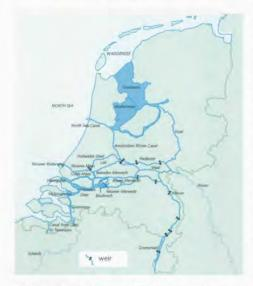
Water distribution over the lower rivers is regulated with weirs and sluices.
