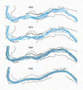
Normalisation of the river Waal in the 18th century. The width of the main channel was reduced from more than 500 metres to 260 metres, islands and sandbanks were removed, and the banks were protected from erosion by regular arrays of groynes.
