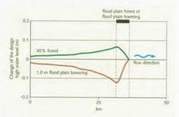
Local measures may have regional impact. Reforestation leads to higher floodwater levels, whilst lowering the embanked flood plain reduces them. The effects of measures taken within a single floodplain section can be observed over a much longer stretch in the upstream direction.
