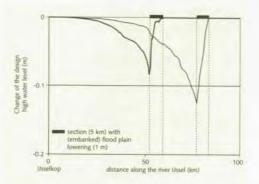
One Rhine branch, different effects. Even along a single river, reaches with wide and narrow floodplains occur, resulting in varying flow velocities along the river stretch. As a result, the same measure will have a different effect on the flood water levels on different locations.
