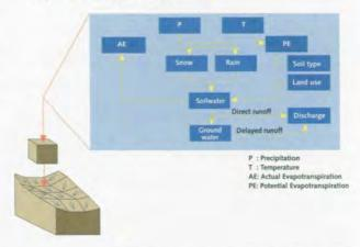
The effect of climate change on the river discharge can be determined with hydrological models which simulate the hydrologic cycle.
