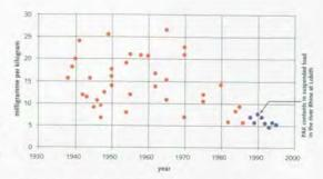
Contents of different PAK's in sediment cores from IJsselmeer and the Rhine.
