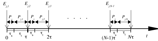
Figure 2.2: Energy-harvesting and energy-consumption models for user j \in \{1, 2\} .
