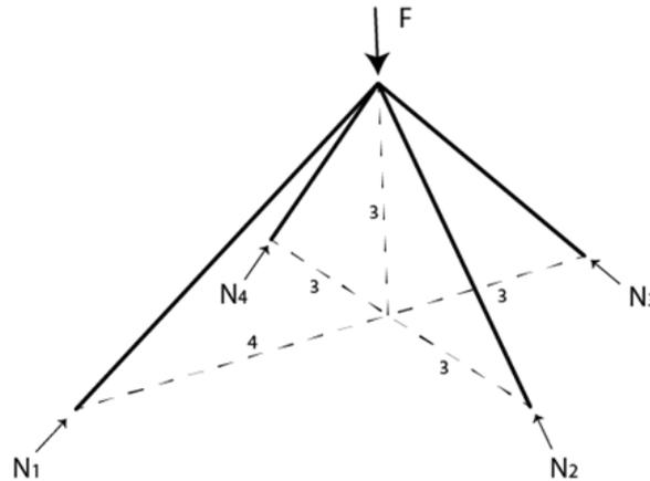
Figure 26 Statically indeterminate structure (Own image)
