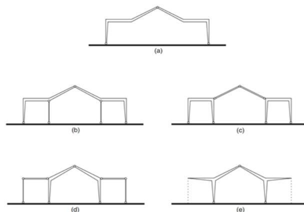
Figure 2 Different structural layouts affect how spaces are read. (Charleson, 2005)
