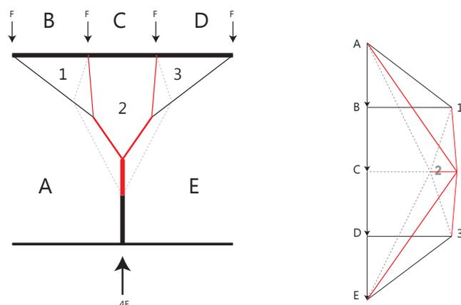
Figure 19 Moving point of branching (own image)
