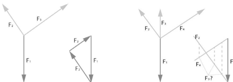
Figure 14 Head tail method (a) and a statically indeterminate configuration(b) (van Dijk, 2014)
