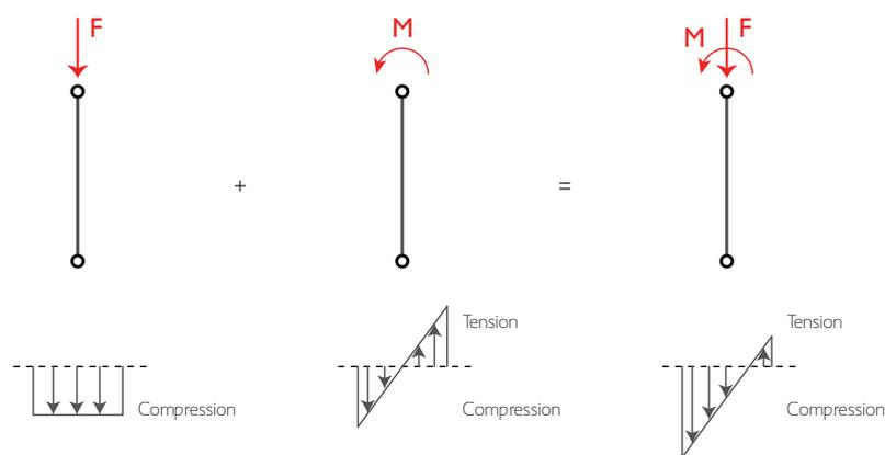
Figure 8 Structural behavior of normal forces and bending moments (own image)
