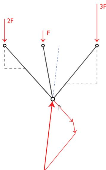
Figure 45 Closed force polygon, reaction force (Own image)
