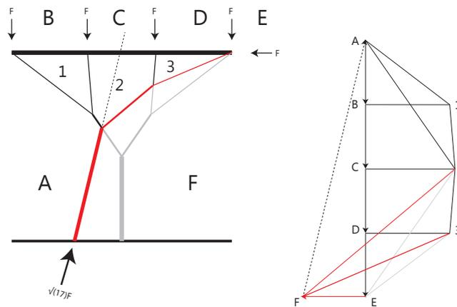
Figure 20 External force on branching structure (own image)
