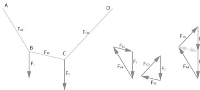
Figure 15 Multiple forces on a cable in equilibrium (Dool, 2012)
