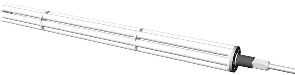
Figure 77 Multiple spacers along the member length to decrease buckling length (Own image)
