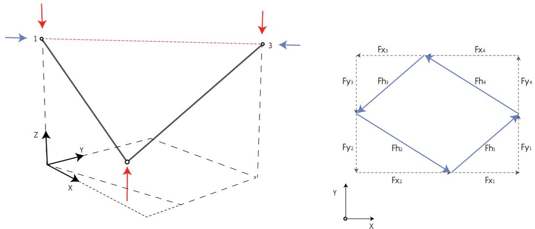
Figure 33 Equality of opposite forces and horizontal closed force polygon (Own image)
