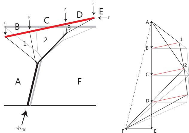
Figure 21 Tilting of the top surface. (own image)
