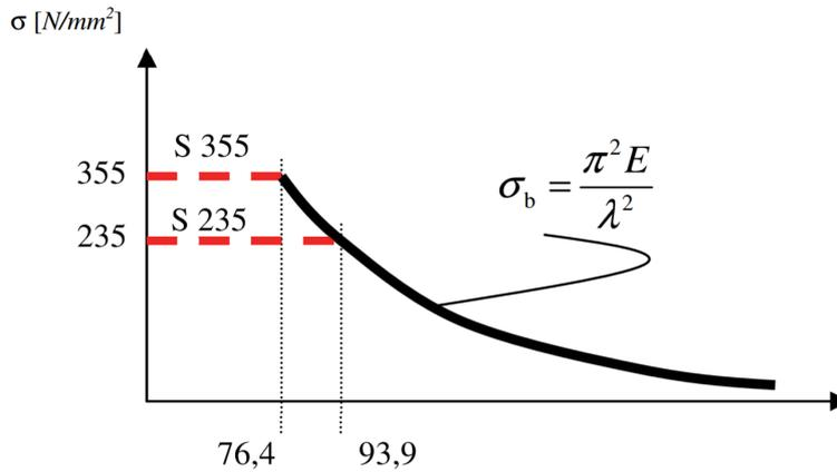
Figure 58 Slenderness (x-axis) and the maximum stress (y-axis)
