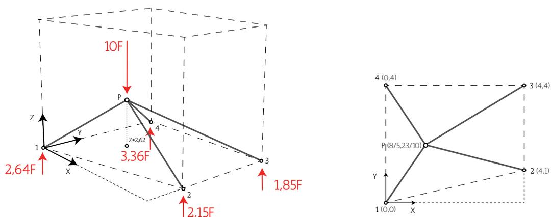
Figure 41 Solution of minimal complementary energy (Own image)
