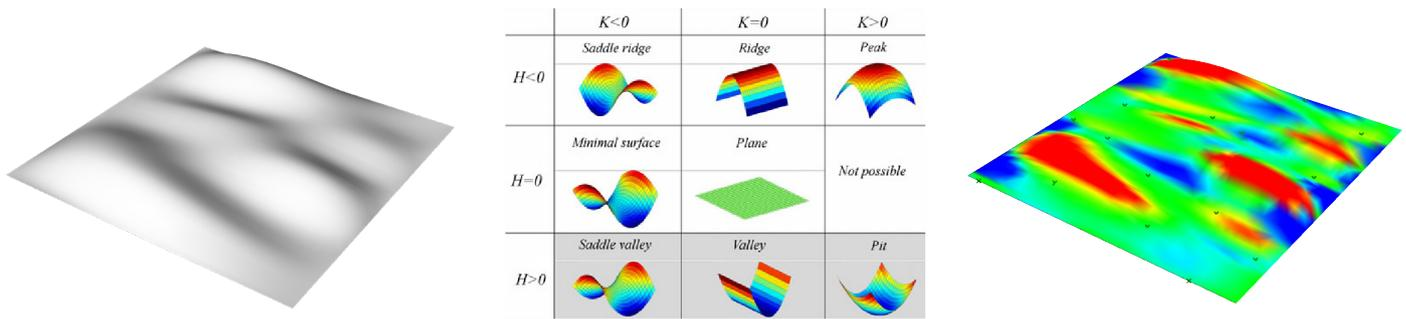
Figure 69 Surface curvature analysis
