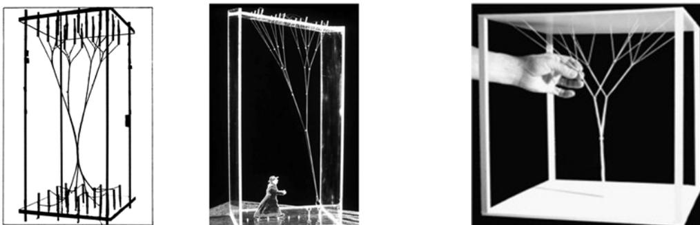
Figure 10 Different model studies of branching structures.
