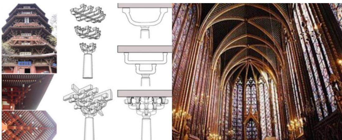
Figure 4 (a) dougong technique and (b) a gothic ribbed vault. (Rian & Sassone, 2014)
