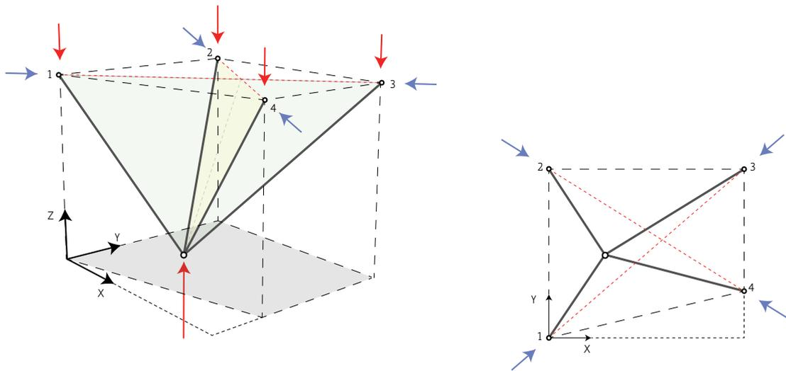
Figure 32 Horizontal forces due to inclination of members (Own image)
