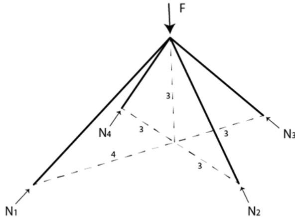
Figure 23 Statically indeterminate system (Own image)
