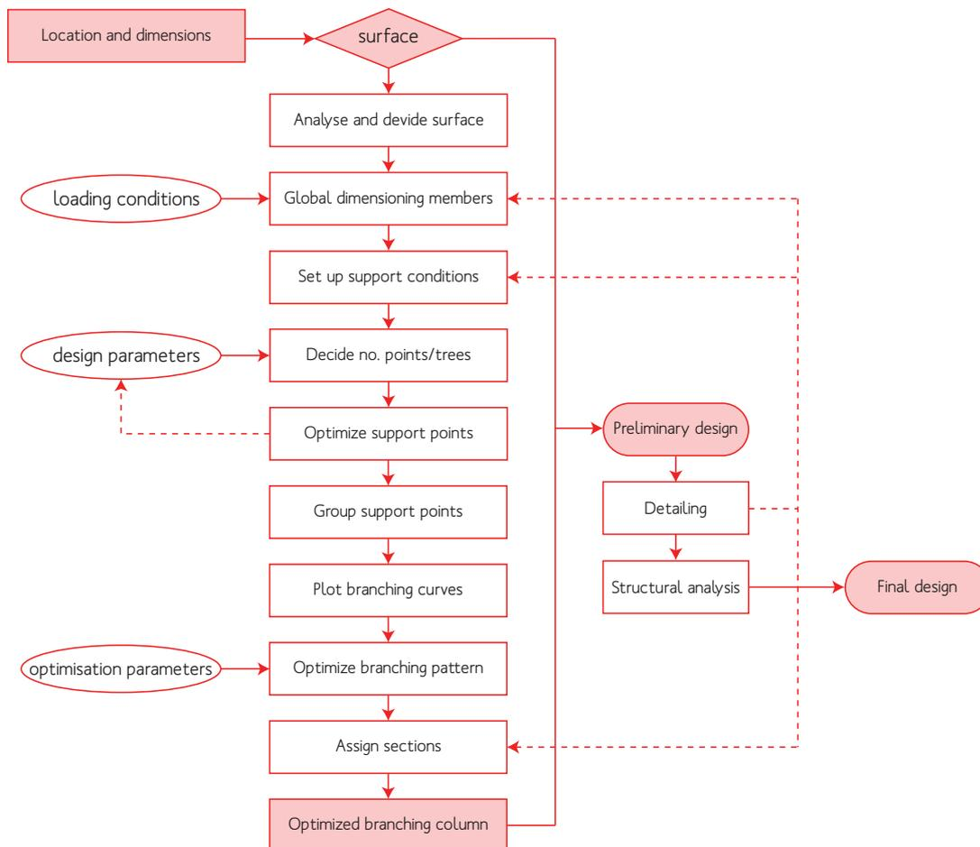
Figure 80 Design method derived from research (Own image)
