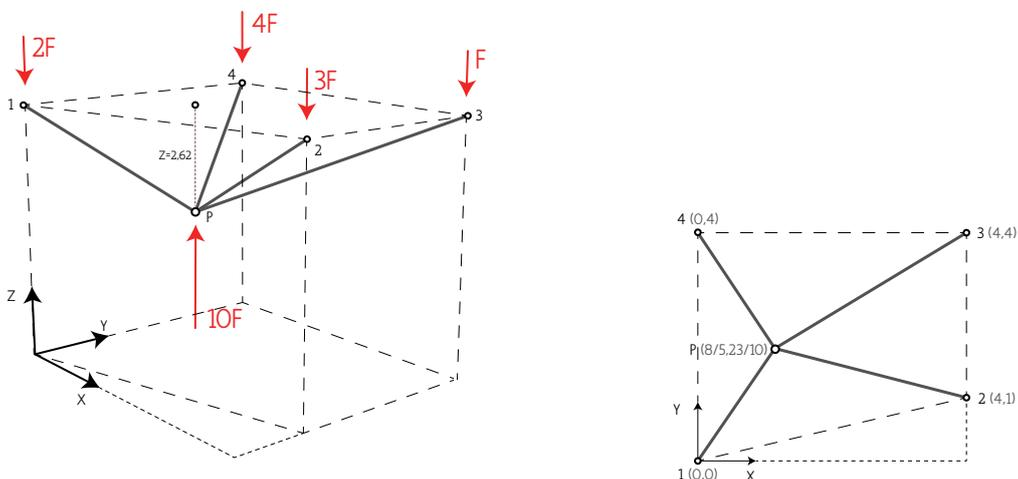
Figure 39 Optimal height branching point (Own image)
