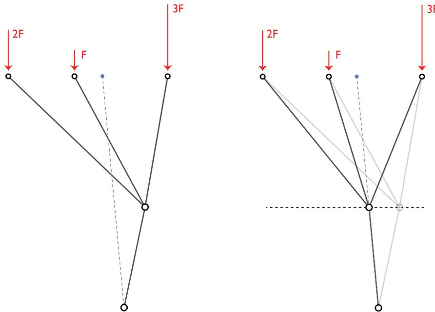
Figure 48 Move branching point to exclude bending moments (Own image)
