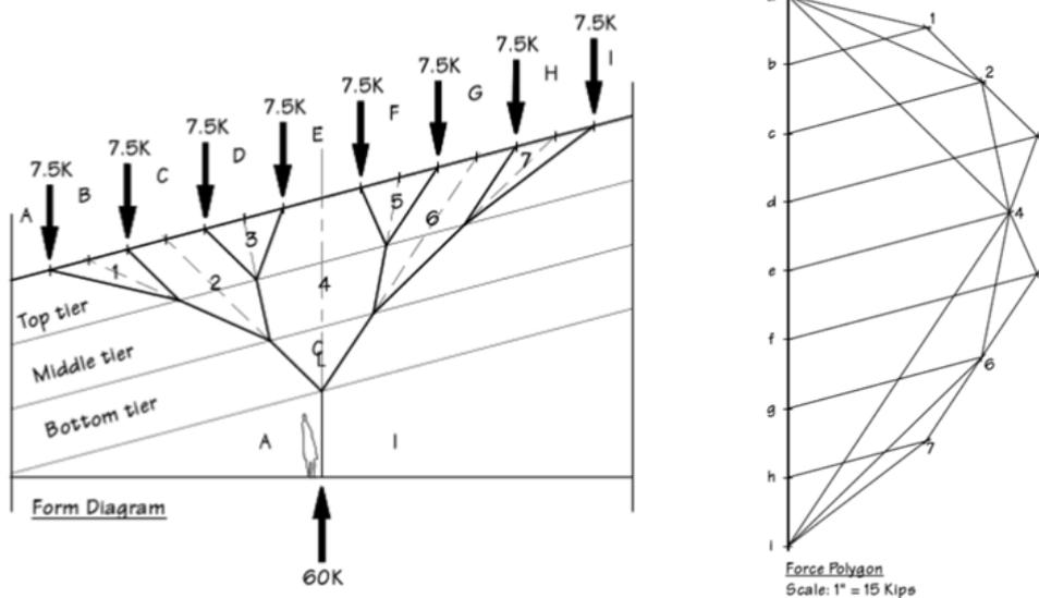
Figure 17 Form and Force (cremona) diagram of a branching structure (Allen & Zalewsky, 2012)
