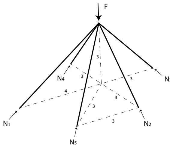
Figure 24 2 times statically indeterminate structure (Own image)
