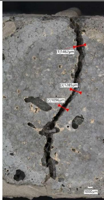
Figure 125 - Photomicrograph of mortar sample P2 showing crack. Scale: 1000µm
