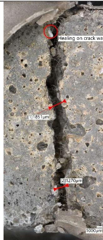
Figure 131 - Photomicrograph of mortar sample PLA4 showing crack. Scale: 1000µm
