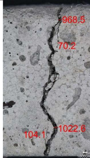
Figure 83 - Photomicrograph of mortar sample PLA2 showing crack. Scale: 1000µm
