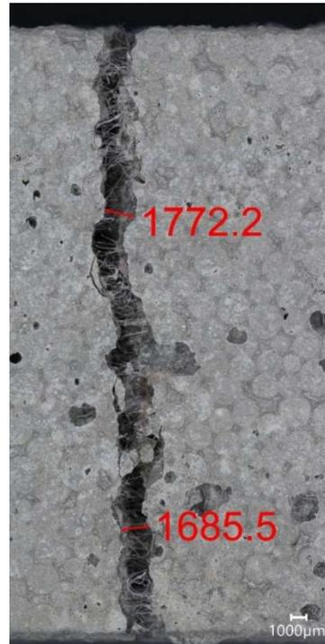
Figure 85 - Photomicrograph of mortar sample PLA4 showing crack. Scale: 1000µm
