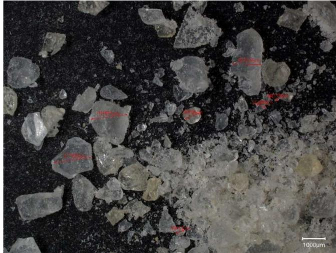
Figure 16- Measurements of PLA capsules. Scale- 1000µm
