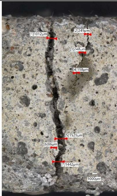
Figure 128 - Photomicrograph of mortar sample PLA1 showing crack. Scale: 1000µm
