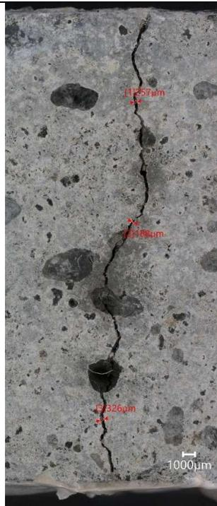
Figure 102 - Photomicrograph of mortar sample P3 showing crack. Scale: 1000µm
