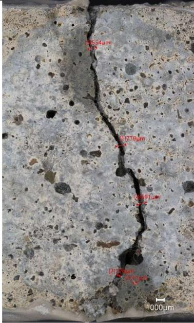
Figure 115 -Photomicrograph of mortar sample A1 showing crack. Scale: 1000µm
