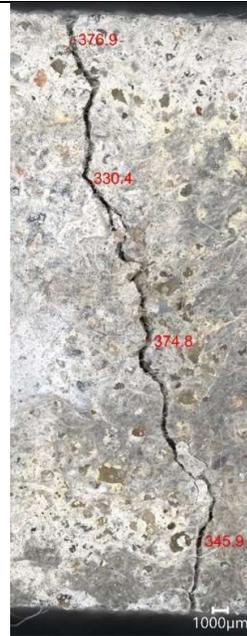
Figure 75-Photomicrograph of mortar sample E2 showing crack. Scale: 1000µm
