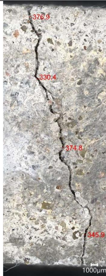
Figure 97-Photomicrograph of mortar sample E2 showing crack. Scale: 1000µm
