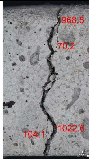
Figure 61 - Photomicrograph of mortar sample PLA2 showing crack. Scale: 1000µm
