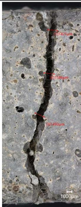
Figure 106 - Photomicrograph of mortar sample PLA3 showing crack. Scale: 1000μm
