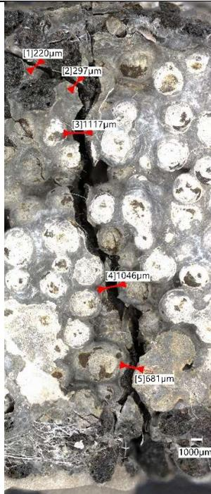
Figure 135 - Photomicrograph of mortar sample EC3 showing crack. Scale: 1000µm
