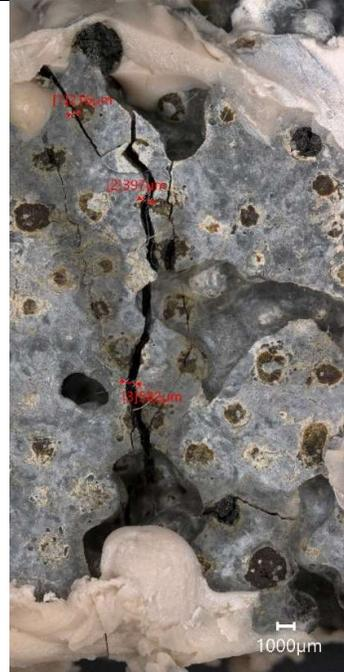
Figure 111 - Photomicrograph of mortar sample EC2 showing crack. Scale: 1000µm
