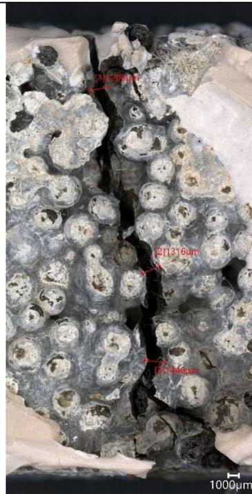
Figure 113 -Photomicrograph of mortar sample EC4 showing crack. Scale: 1000µm
