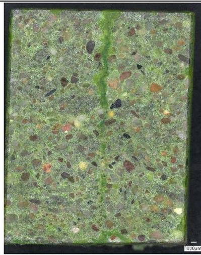
Figure 154 - Photomicrograph of polished sample E1 showing crack. Scale: 1000µm
