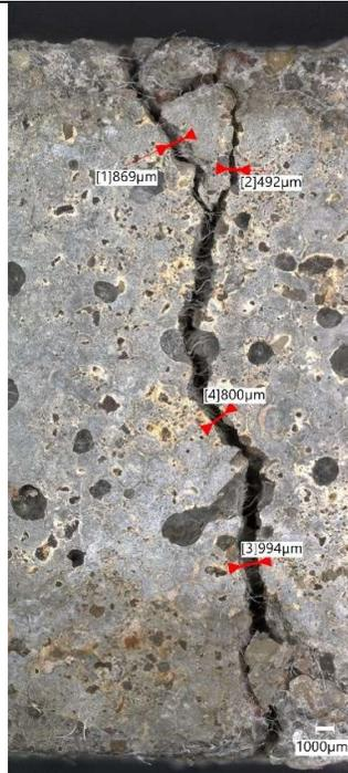
Figure 124 - Photomicrograph of mortar sample P1 showing crack. Scale: 1000µm
