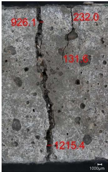
Figure 60 - Photomicrograph of mortar sample PLA1 showing crack. Scale: 1000µm
