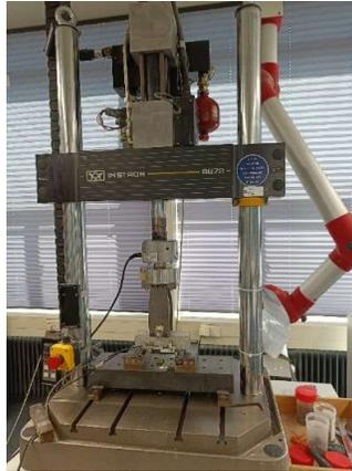
Figure 30 -Testing sample in 4-point bending
