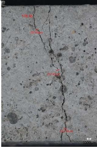
Figure 86 -Photomicrograph of mortar sample PLA5 showing crack. Scale: 1000µm
