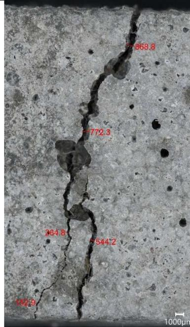
Figure 71 -Photomicrograph of mortar sample A2 showing crack. Scale: 1000µm
