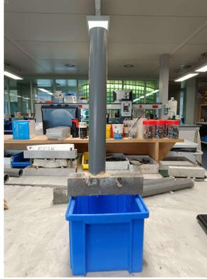
Figure 31 - Setup for permeability test
