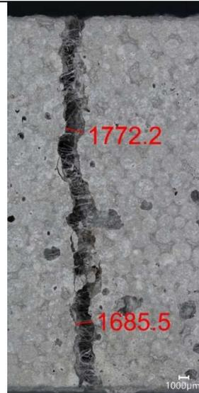
Figure 63 - Photomicrograph of mortar sample PLA4 showing crack. Scale: 1000µm
