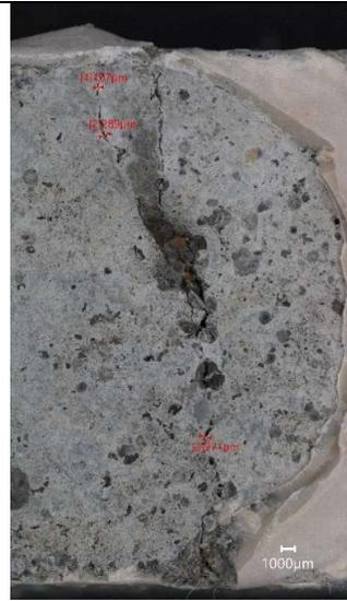
Figure 109 -Photomicrograph of mortar sample PLA5 showing crack. Scale: 1000µm
