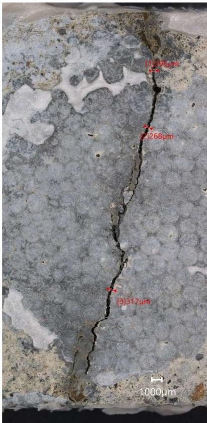
Figure 117-Photomicrograph of mortar sample A3 showing crack. Scale: 1000µm
