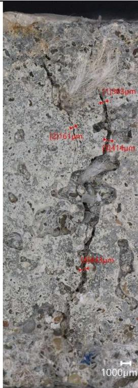
Figure 123-Photomicrograph of mortar sample E4 showing crack. Scale: 1000µm
