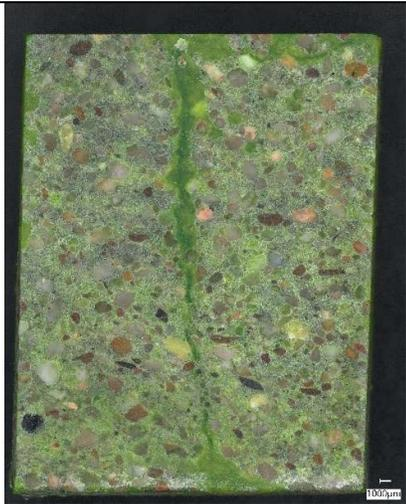
Figure 153 - Photomicrograph of polished sample E1 showing crack. Scale: 1000µm
