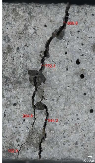
Figure 93 -Photomicrograph of mortar sample A2 showing crack. Scale: 1000µm
