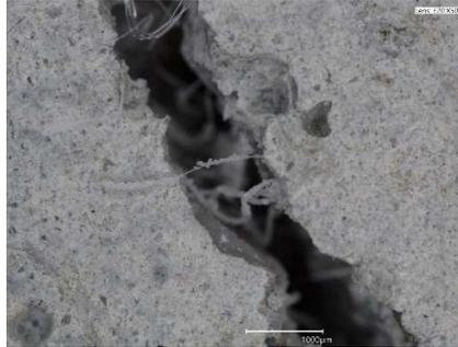
*Figure 55 -Photomicrograph of precipitate along the fiber across the crack. Scale: 1000µm*
