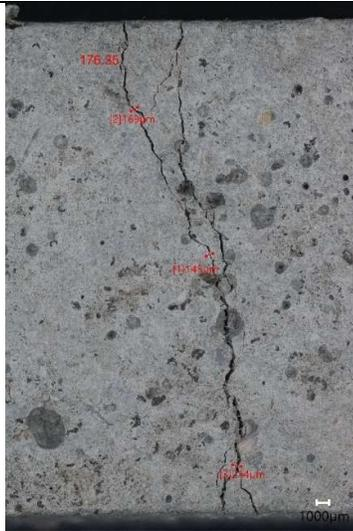
Figure 64 -Photomicrograph of mortar sample PLA5 showing crack. Scale: 1000µm
