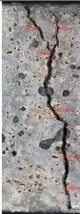
Figure 100 - Photomicrograph of mortar sample P1 showing crack. Scale: 1000µm
