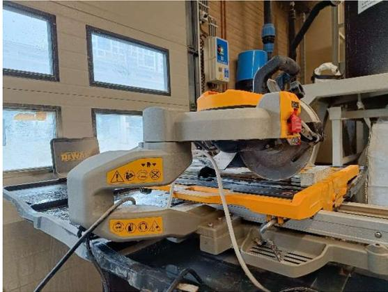
Figure 28 -Saw for cutting the prism samples
