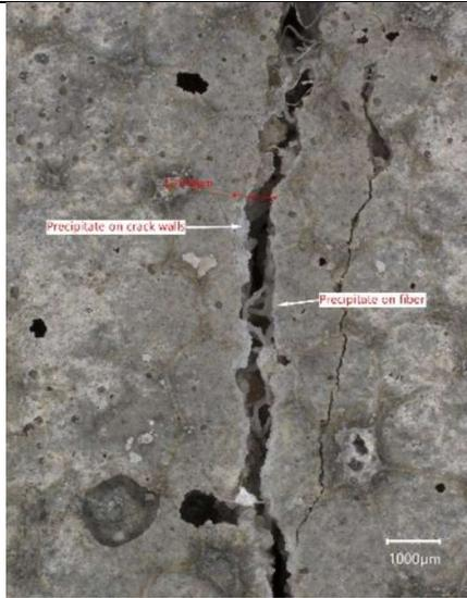
Figure 108 – PLA 4 sample showing precipitate along the crack Scale: 1000µm
