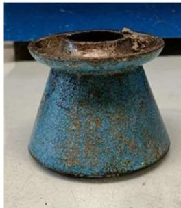
*Figure 26 - Slump Cone*
