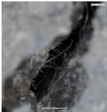
Figure 52 -Photomicrograph of fiber pullout across the crack. Scale: 1000µm
