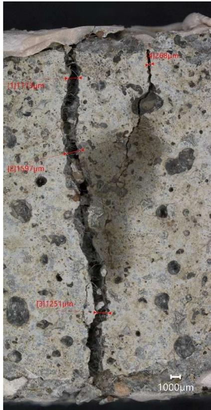
Figure 104 - Photomicrograph of mortar sample PLA1 showing crack. Scale: 1000μm
