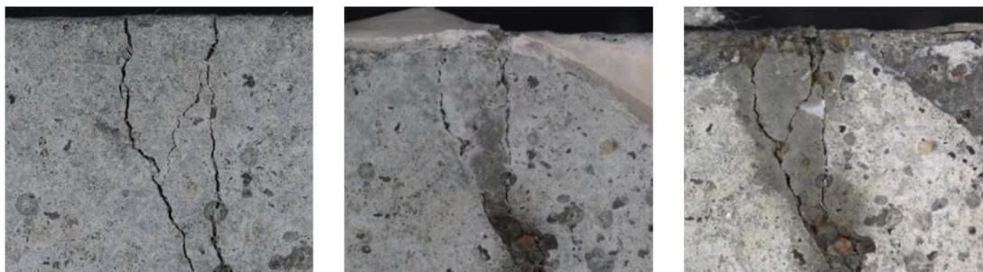
Figure 35 -Photomicrographs of sample PLA5 (Type 2) at cracking (left), 1 month healing (middle), 2 months healing (right). Healing can be seen in the crack. Scale: 1000 µm (0.222 pixels/micron)
