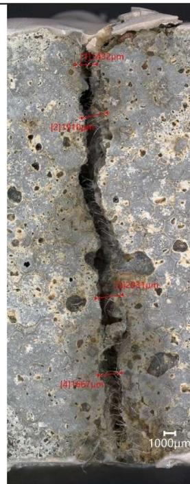
Figure 107 - Photomicrograph of mortar sample PLA4 showing crack. Scale: 1000μm
