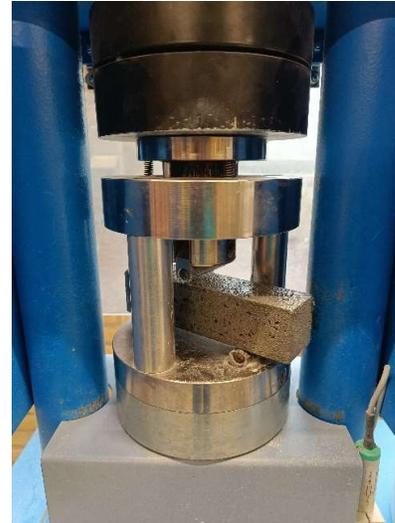
Figure 29 -Type 2 specimen undergoing flexure strength test
