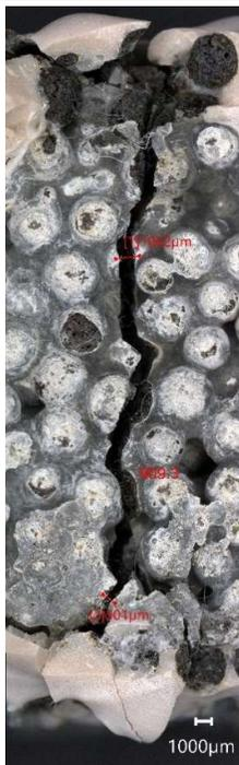
Figure 112- Photomicrograph of mortar sample EC3 showing crack. Scale: 1000µm
