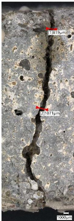
Figure 130 - Photomicrograph of mortar sample PLA3 showing crack. Scale: 1000µm
