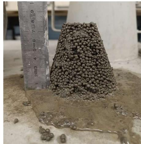
Figure 33 - Consistency of Type 3 Mix showing segregation
