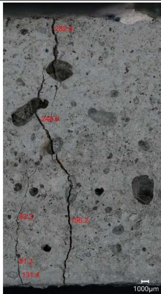
Figure 98-Photomicrograph of mortar sample E3 showing crack. Scale: 1000µm
