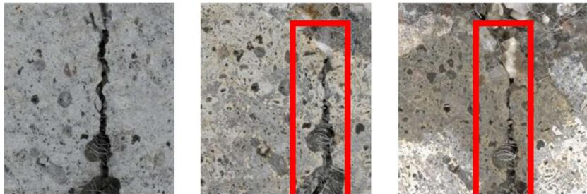
Figure 38-Photomicrographs of sample E1 (Type 5) at cracking (left), 1 month healing (middle), 2 months healing (right). Healing can be seen in the crack. Scale: 1000 µm
