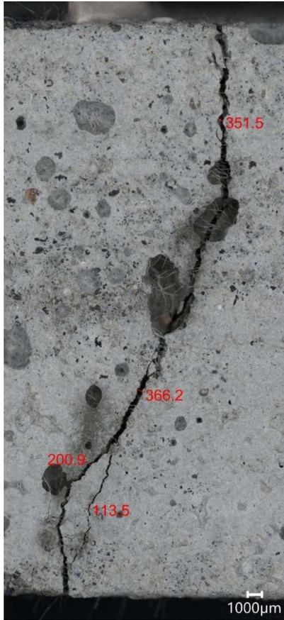
Figure 96 -Photomicrograph of mortar sample E1 showing crack. Scale: 1000µm
