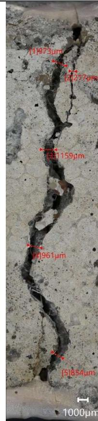
Figure 105 - Photomicrograph of mortar sample PLA2 showing crack. Scale: 1000μm
