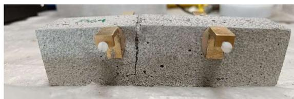
Figure 34-Crack in Type 2 sample with some visible crack bridging
