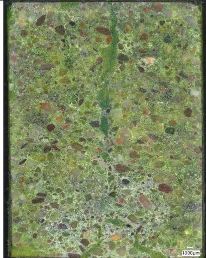
Figure 148- Photomicrograph of polished sample PLA1 showing crack. Scale: 1000µm
