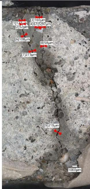
Figure 132 -Photomicrograph of mortar sample PLA5 showing crack. Scale: 1000µm
