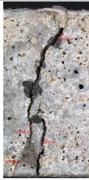
Figure 116 -Photomicrograph of mortar sample A2 showing crack. Scale: 1000µm
