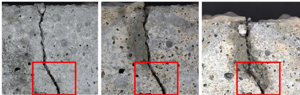
Figure 37-Photomicrographs of sample A1(Type 4) at cracking (left), 1 month healing (middle), 2 months healing (right). Healing can be seen in the crack. Scale: 1000 µm
