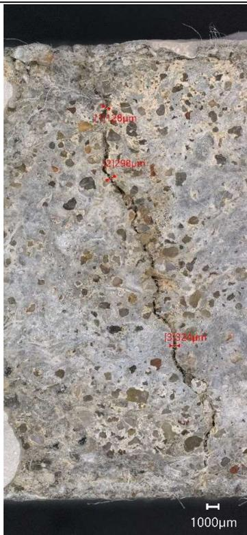
Figure 121- Photomicrograph of mortar sample E2 showing crack. Scale: 1000µm
