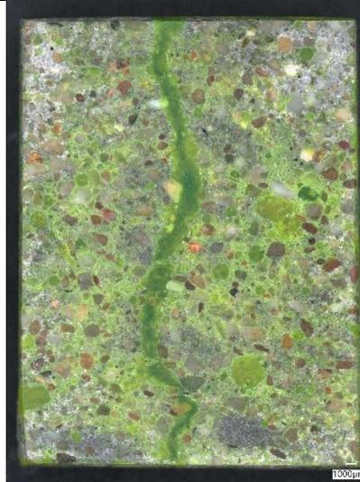
Figure 152 - Photomicrograph of polished sample A1 showing crack. Scale: 1000µm
