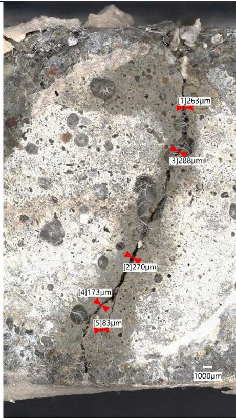
Figure 141 -Photomicrograph of mortar sample E1 showing crack. Scale: 1000µm
