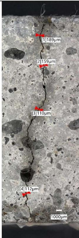
Figure 126 - Photomicrograph of mortar sample P3 showing crack. Scale: 1000µm
