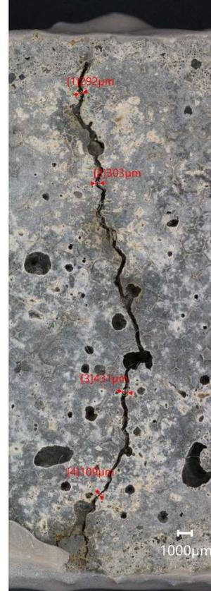
Figure 118-Photomicrograph of mortar sample A4 showing crack. Scale: 1000µm
