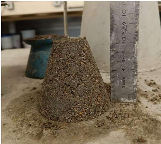
Figure 32 - Consistency of Type 2 mix
