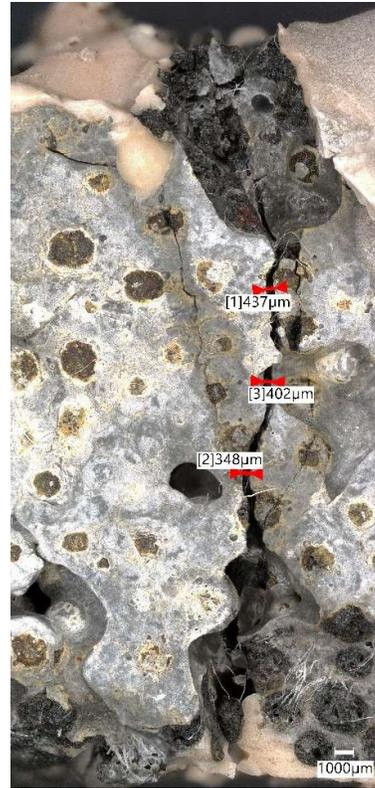
Figure 134 - Photomicrograph of mortar sample EC2 showing crack. Scale: 1000µm
