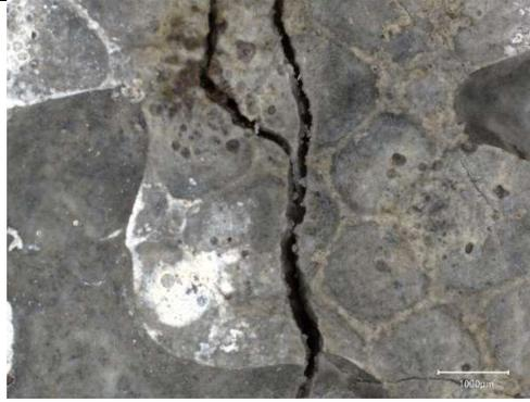
*Figure 114- Photomicrograph of left side of mortar sample EC4 showing crack. Scale: 1000μm*
