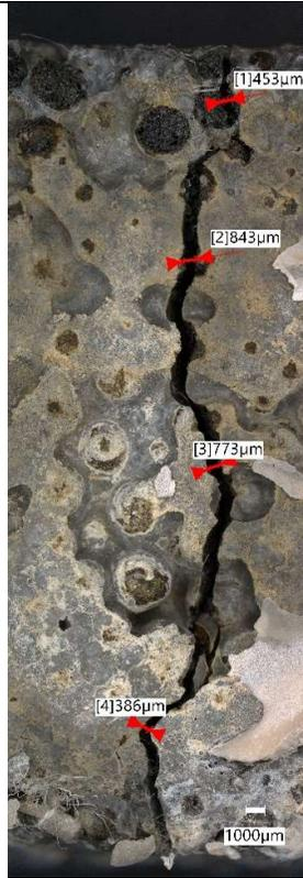
Figure 133 -Photomicrograph of mortar sample EC1 showing crack. Scale: 1000µm
