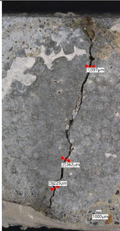
Figure 139-Photomicrograph of mortar sample A3 showing crack. Scale: 1000µm
