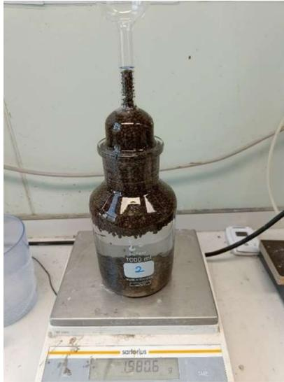
Figure 19 - Pycnometer after 24 hours
