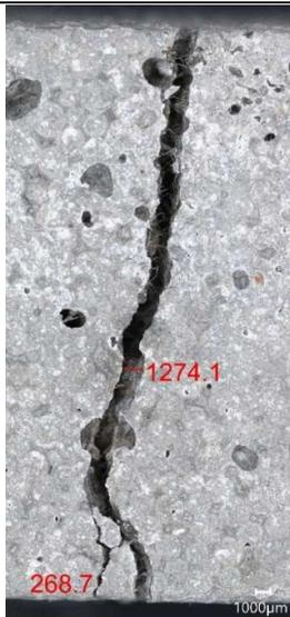
Figure 62 - Photomicrograph of mortar sample PLA3 showing crack. Scale: 1000µm
