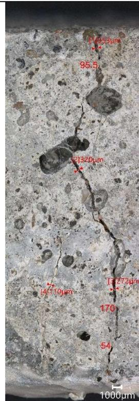
Figure 122-Photomicrograph of mortar sample E3 showing crack. Scale: 1000µm
