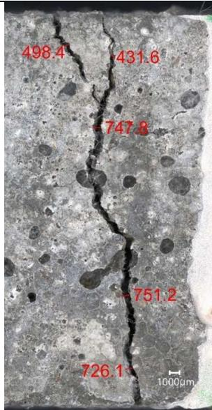
Figure 78 - Photomicrograph of mortar sample P1 showing crack. Scale: 1000µm
