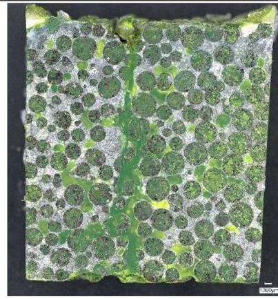
Figure 150 -Photomicrograph of polished sample EC3 showing crack. Scale: 1000µm
