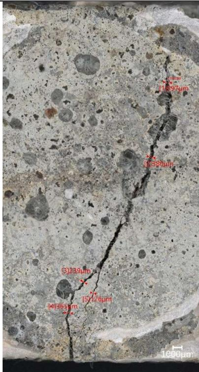
Figure 119 -Photomicrograph of mortar sample E1 showing crack. Scale: 1000µm
