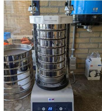
Figure 17 - Sieving of expanded clay particles in a sieve shaker.
