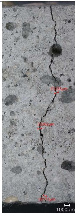
Figure 80 - Photomicrograph of mortar sample P3 showing crack. Scale: 1000µm
