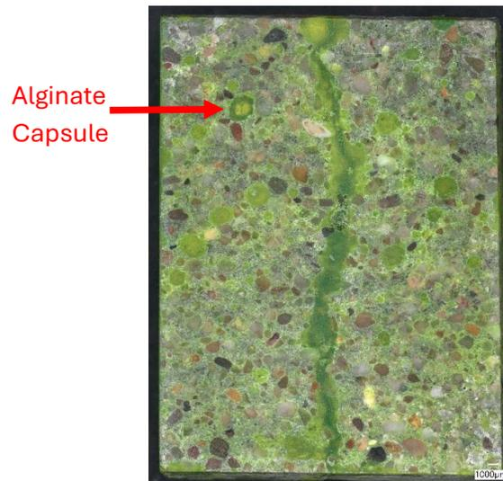
Figure 50 - Photomicrograph of polished sample A1 showing crack. Scale: 1000µm
