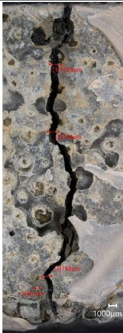
Figure 110 -Photomicrograph of mortar sample EC1 showing crack. Scale: 1000µm
