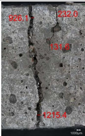
Figure 82 - Photomicrograph of mortar sample PLA1 showing crack. Scale: 1000µm
