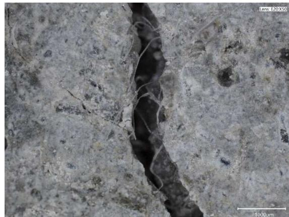
Figure 53 - Photomicrograph of elongation of fibers across the crack. Scale: 1000µm
