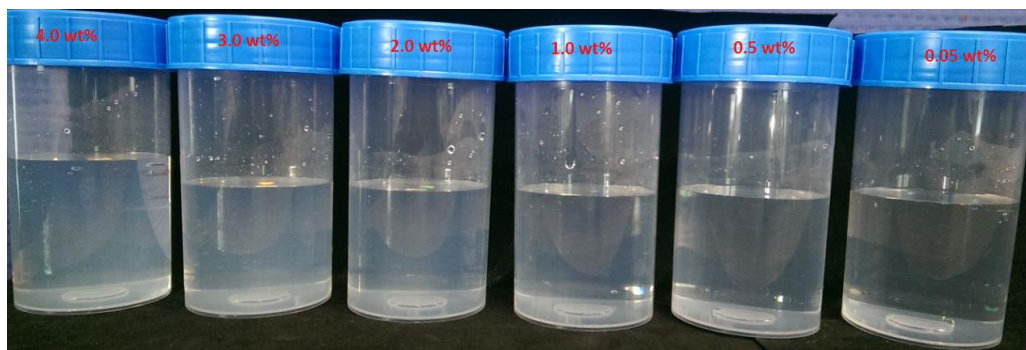
Figure A.1: Samples of GPTMS modified silica NPs at different concentrations dispersed in Brine2015; from right to left: 0.05, 0.5, 1.0, 2.0, 3.0 and 4 wt%
