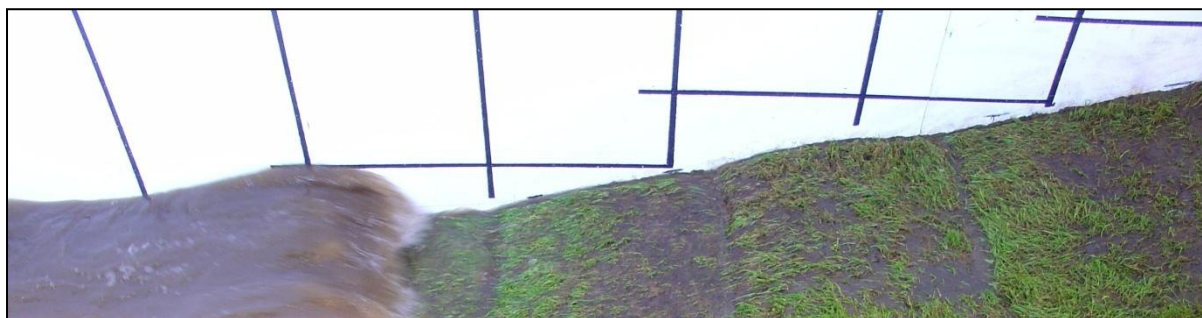
Figure A-8: Grid on the flume wall.
