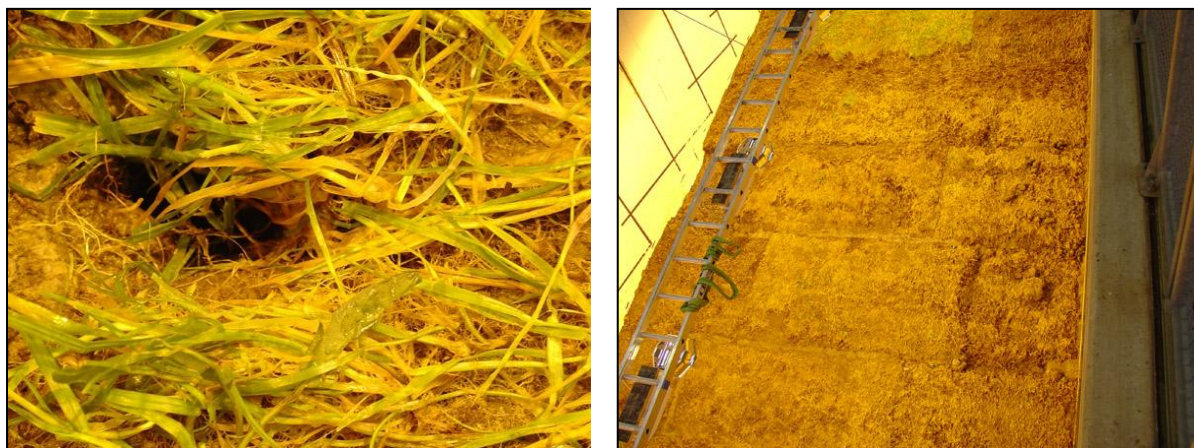
Figure A-13: Small holes were formed during the tests (left). Grass cover in breaker zone was less green than lower parts of the outer slope (right). [Piontkowitz et al. 2009]
