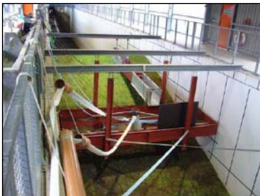
Figure A-5: Overtopping container with inlet and hose system. [Piontkowitz et al. 2009]
