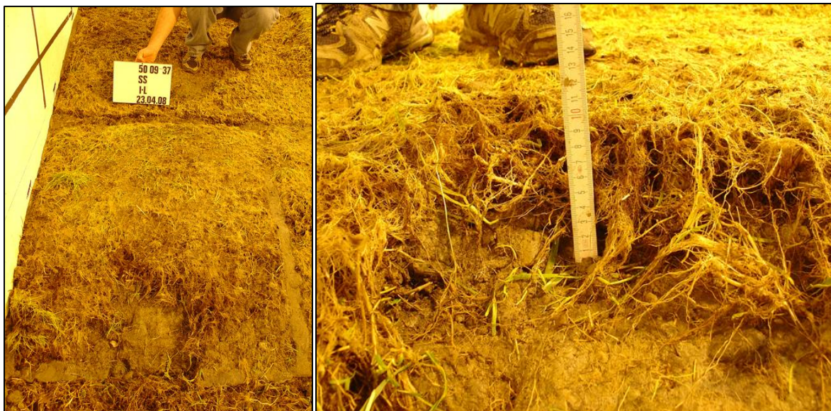
Figure A-17: Erosion of grass mat I-L near the lower joint (left). Depth of the erosion hole (right).
