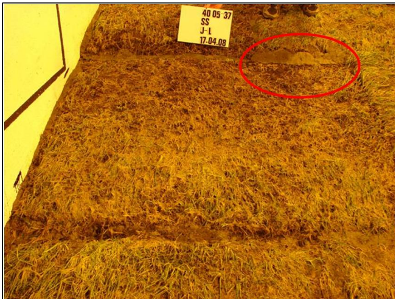
Figure A-15: Erosion at J-L after test 16040801, clay placed on the joints was eroded.
