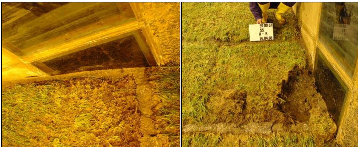
Figure A-10: Grass before wave impact damage (left), first damage after wave impact (right).
