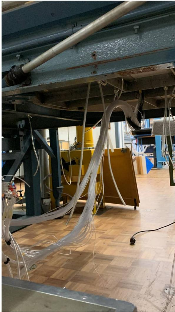
**Figure 4.7:** Tubes exiting the model for measuring pressure distribution
