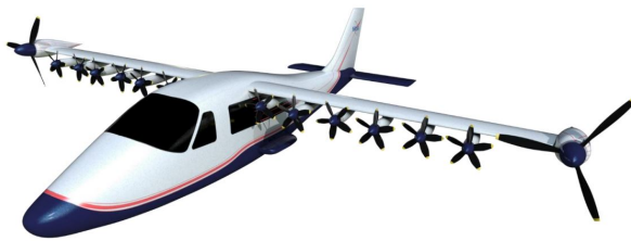
Figure 1.8: Wingtip-mounted propeller concept by NASA; X-57[43].
