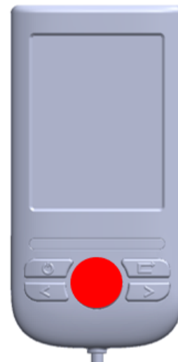
Fig. 19: Remote controller that implemented an emergency button (shown in red) for deactivating the system when needed.
