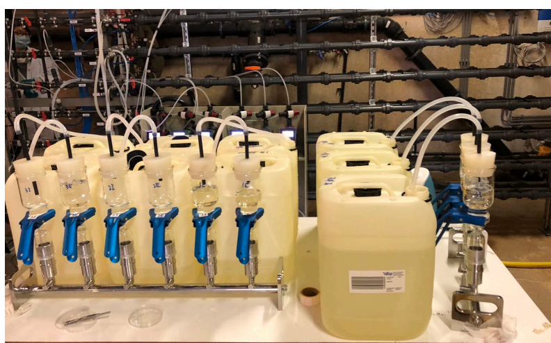
Figure 3.2 Continuous water filtration setup
