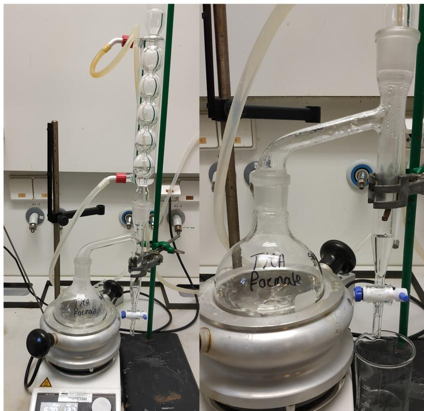
Figure 7.4: distillation column for decomposition of TMA formate.
