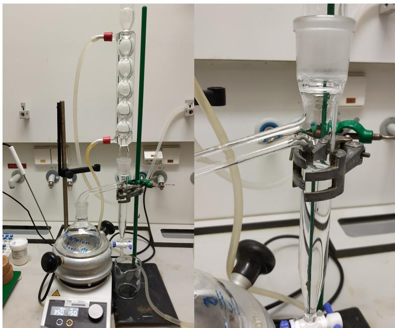
Figure 3.5: Lab distillation column for decomposition of ammonium formate.
