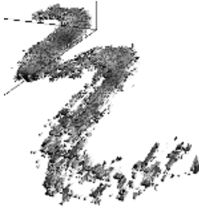
Figure 6-14: resulting \alpha -complex of the L8 river, 3D oblique view. T indicate the typical size of tetrahedral elements, the figure shows a slightly exploded view. The total number of tetrahedra amounts to 38835.
