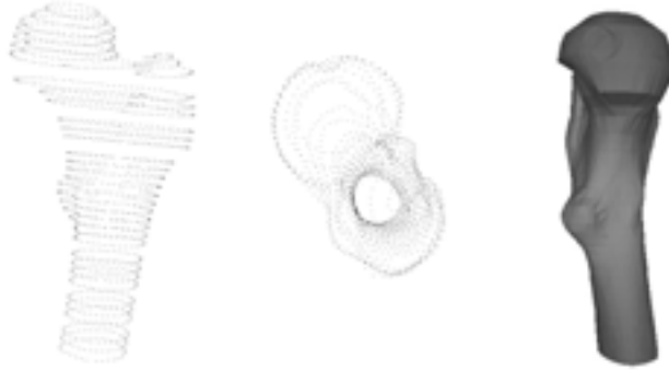
Figure 3-7: Contour sampling data point set of the femur, the upper extreme of the thy bone. The \alpha -complex geometric model is shown at the right (contour data obtained form the organ data base, Tel Aviv university, Gill Barequet).
