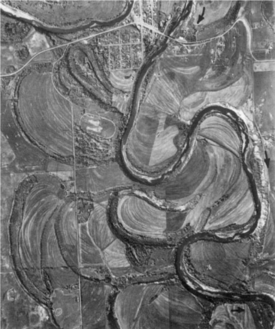
Figure 6–25: Example of the complex, partly labyrinthine, partly jig-saw morphology of a meandering river system. Picture shows a 2.3 \times 2.6 km area of the Millhako river, Alberta, Canada. Observe the frequently reworked depositions (scrollbars) on the river banks at the inner bends. Also the clay-/mud-filled “dead” river channels, abandoned after a short cutting “neck chute”. The point bars form a labyrinth of permeable flow-channels and are able to trap hydrocarbons. Well design and reservoir simulation is a tedious task in such a reservoir. Photo taken from Allen (1985). Copyright ©: Alberta Energy Company. Reprinted with permission.
