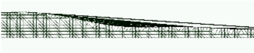
Figure 6–23: fragment of the barchan dune grid at time t = 0 s. The form of the dune is easily recognised in the grid. The grid contains two fans along the top boundary with (necessarily) a elevation of the profile (to the right of the toe of the slip face) separating them. Decreasing \alpha_{\max} a bit will easily remove the slivers adjacent to the slip face.
