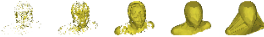
Figure 1–5: example of an evolving \alpha -complex with \alpha increasing left-to-right: left: \alpha = 3.096634e + 01 , yielding a complex that is little more than just the point set with a few singular edges, gradually developing into right: an overly fat ( \alpha = 1.805128e + 03 ) complex obscuring all the fine details of the face and the neck, almost grown into the convex hull. The most appropriate \alpha for the details of the face is approx. \alpha = 1.444991e + 02 , the value of the central picture (data set by Silicon Graphics, number of points N = 2780 ).
