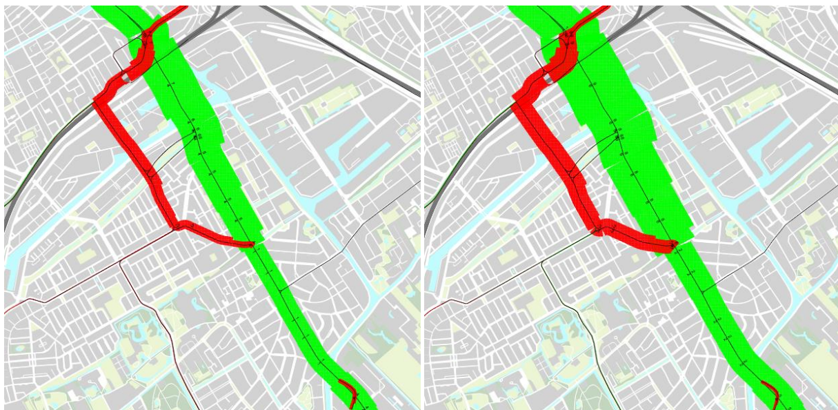
Figure 2. Comparison between predicted ridership effects of a frequency increase without crowding (left) and with crowding (right) effects incorporated (derived from Van Oort et al. 2016)
