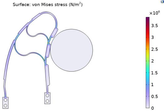
Fig. 2: Von Mises stresses in the compliant finger when actuated in contact with a rigid disc. FEA simulation using COMSOL Multiphysics
