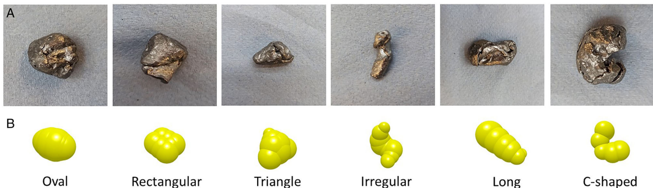
Figure 3. A) Representative shapes of actual steel scrap particles and B) Representations by spherical assembled particles in the discrete element method (DEM) simulations.
