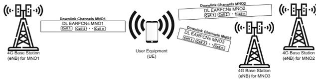
**Fig. 1.** Simplified overview of a Radio Access Network.
