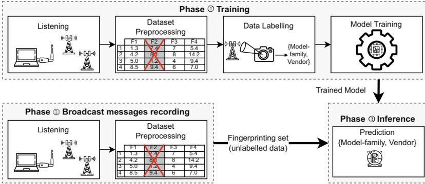
Fig. 2. Fingerprinting phases.
