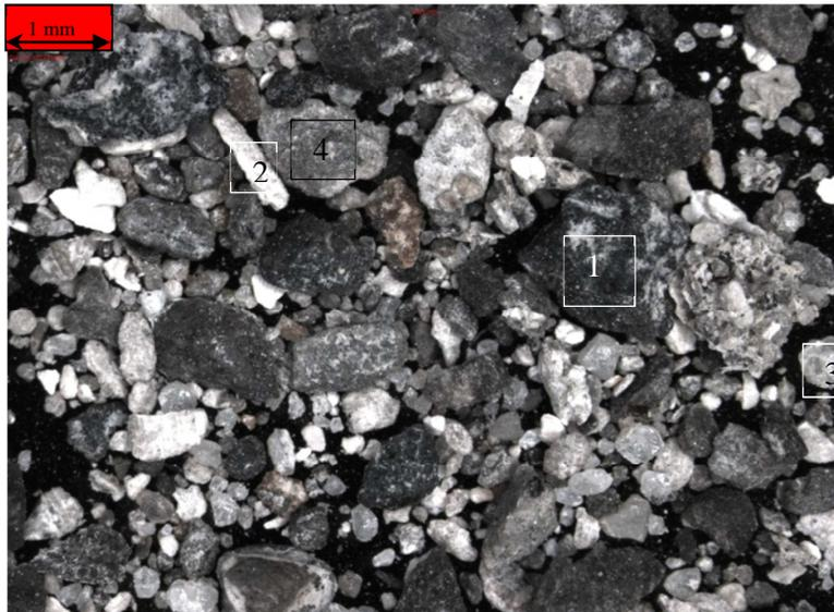
Figure 32 GT01 PNA 2770 fine fraction (0,064mm-1mm) dried cutting sample.
