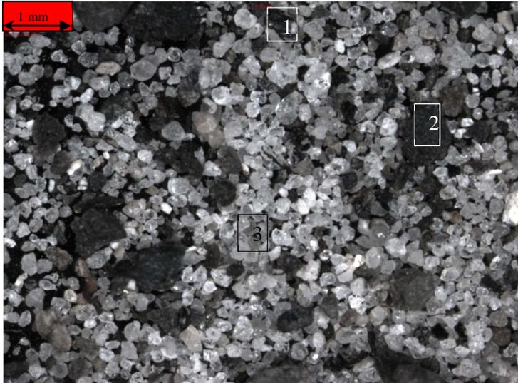
Figure 24GT01 PNA 2752,5 fine fraction (0,064mm-1mm) dried cutting sample.
