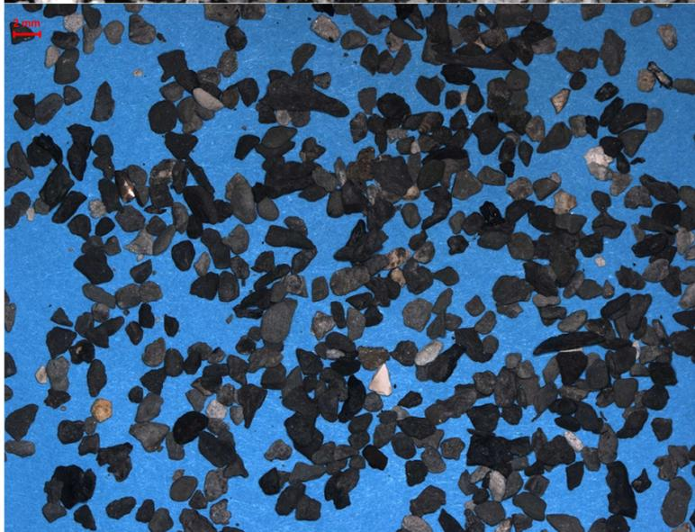
Figure 53 GT01 PNA 2822,5 coarse fraction(1mm-2mm) dried cutting sample. The scale bar in the top left depicts 2mm.
