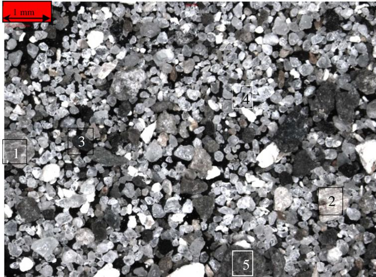
Figure 39 GT01 PNA 2785 fine fraction(0,064mm-1mm) dried cutting sample.
