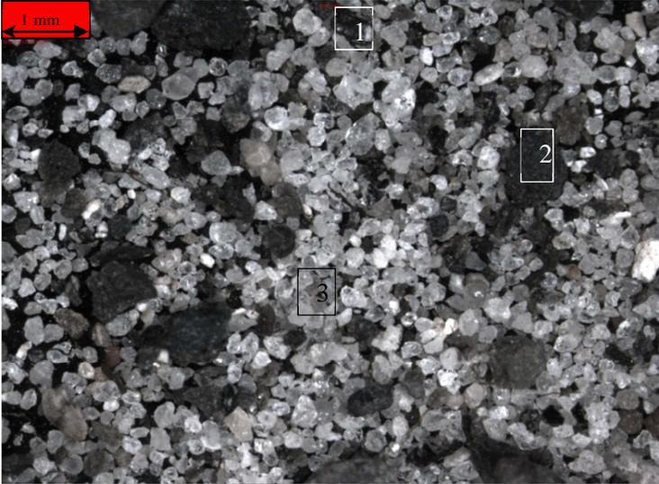
Figure 12GT01 PNA 2752,5 fine fraction (0,064mm-1mm) dried cutting sample. The scale bar in the top left depicts 500microns.
