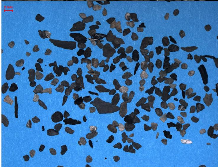
Figure 22GT01 PNA 2742,5 coarse fraction (1mm-2mm) dried cutting sample. The scale bar in the top left depicts 2mm.
