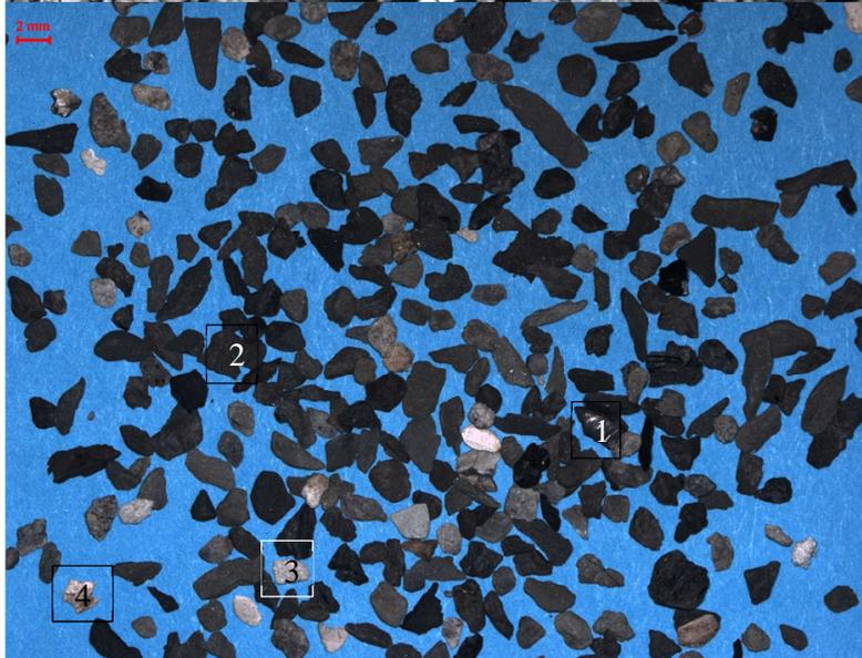
Figure 47 GT01 PNA 2812,5 coarse fraction(1mm-2mm) dried cutting sample. The scale bar in the top left depicts 2mm.
