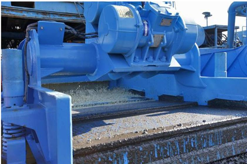
**Figure 3** The Shale shaker in action at the Ammerlaan site
