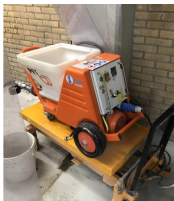
Figure 56. Conveying pump used for 3D printing
