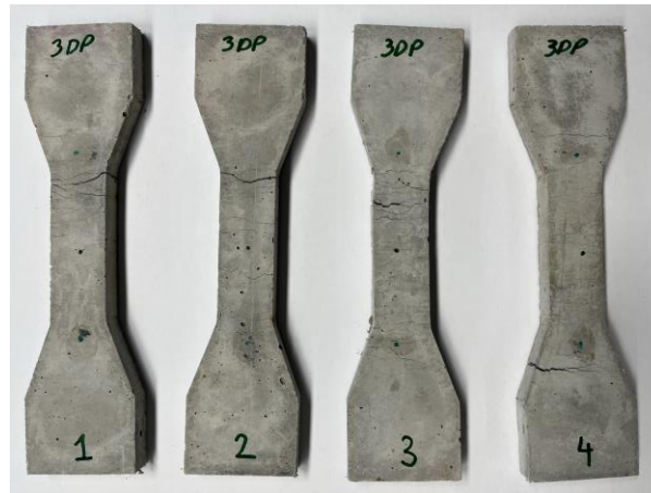
Figure 61. Cracks observed in the dog bone specimens of PE1SF12.5.
