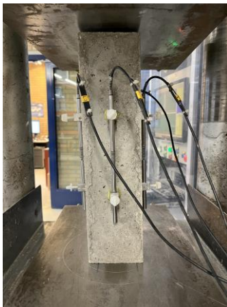
Figure C.2. Non-destructive test setup and parameters used to determine the concrete elastic modulus.
