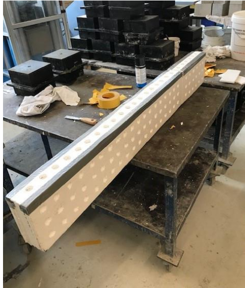
Figure B.1. Inner Styrofoam mould used in the first trial U-shape experiment.
