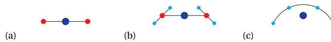
Figure A.10: (a-c) Cross-section of 3D subdivision schemes, the blue dot represents the original spring, the two red dots and the four cyan dots are equivalent to original blue spring, stiffness is equivalent to surface area of dots.
