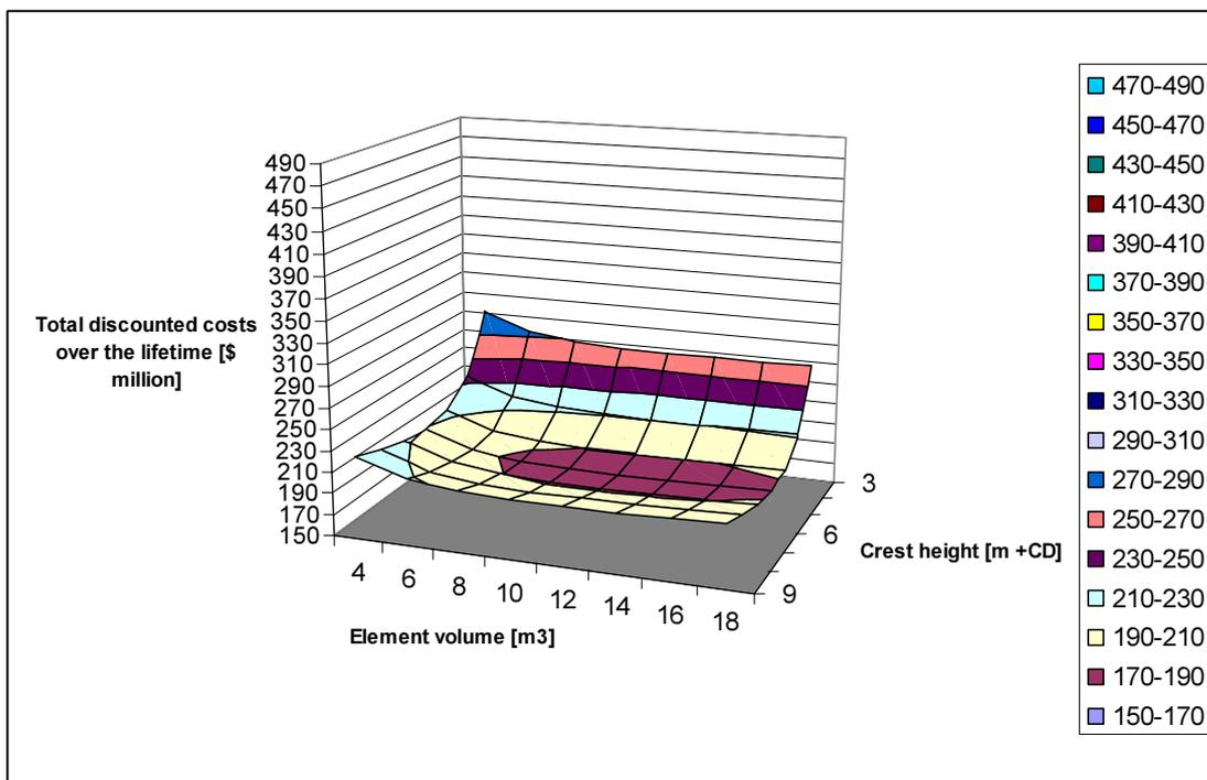
Figure 51 discounted costs over the lifetime without throughput growth rate [\$ million]
