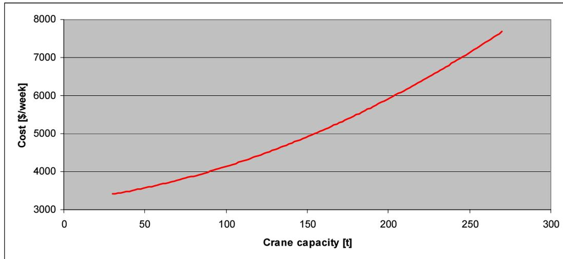
Figure 26 Crane Cost as a function of crane capacity
