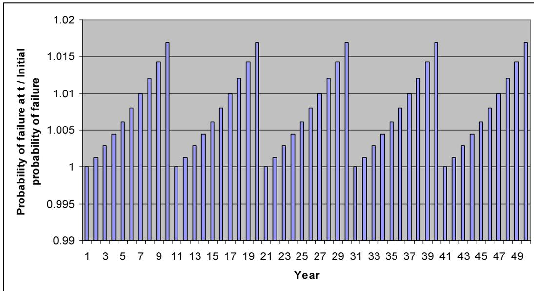
Figure 36 Fictitious probability of collapse for Core-loc® armour
