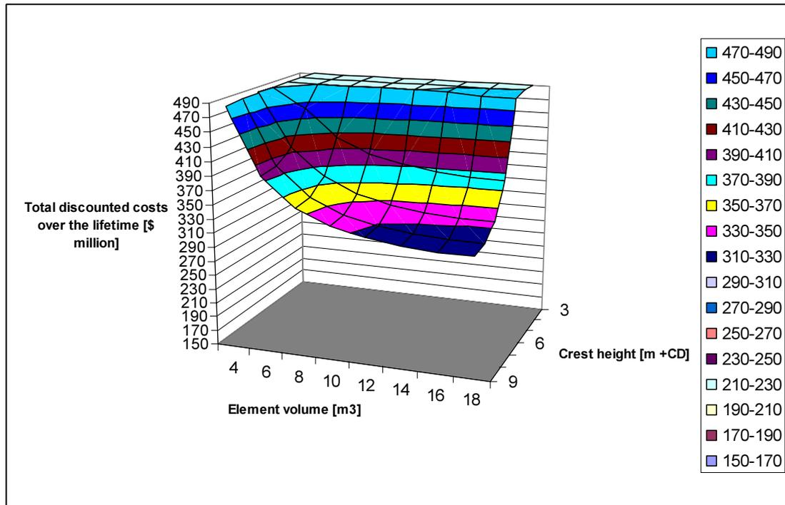
Figure 54 Total discounted costs over the lifetime with a 9% throughput growth rate [\$ million]
