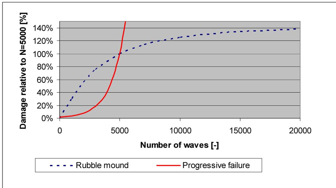
Figure 14 Evolution of damage as a function of time
