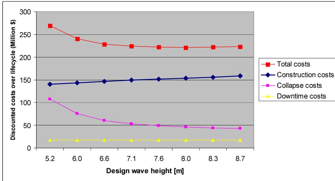
Figure 46 Costs for significant design wave height variation for crest height 7m +CD
