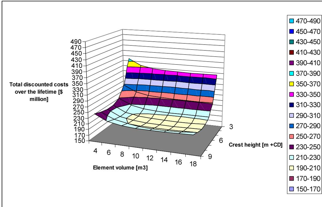
Figure 52 Total discounted costs over the lifetime with a 3% throughput growth rate [\$ million]
