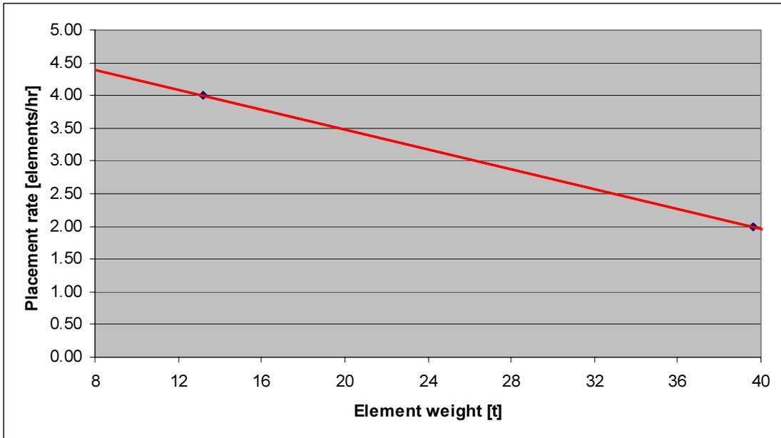
Figure 24 Placement rate as a function of element weight
