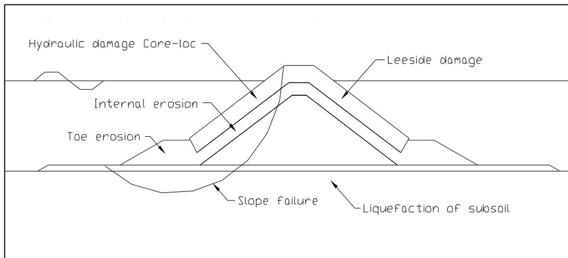
Figure 27 Breakwater failure mechanisms
