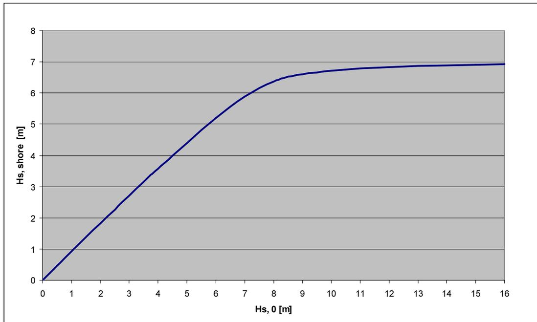
Figure 11 Relation significant deep and shallow wave height at -16 m+CD
