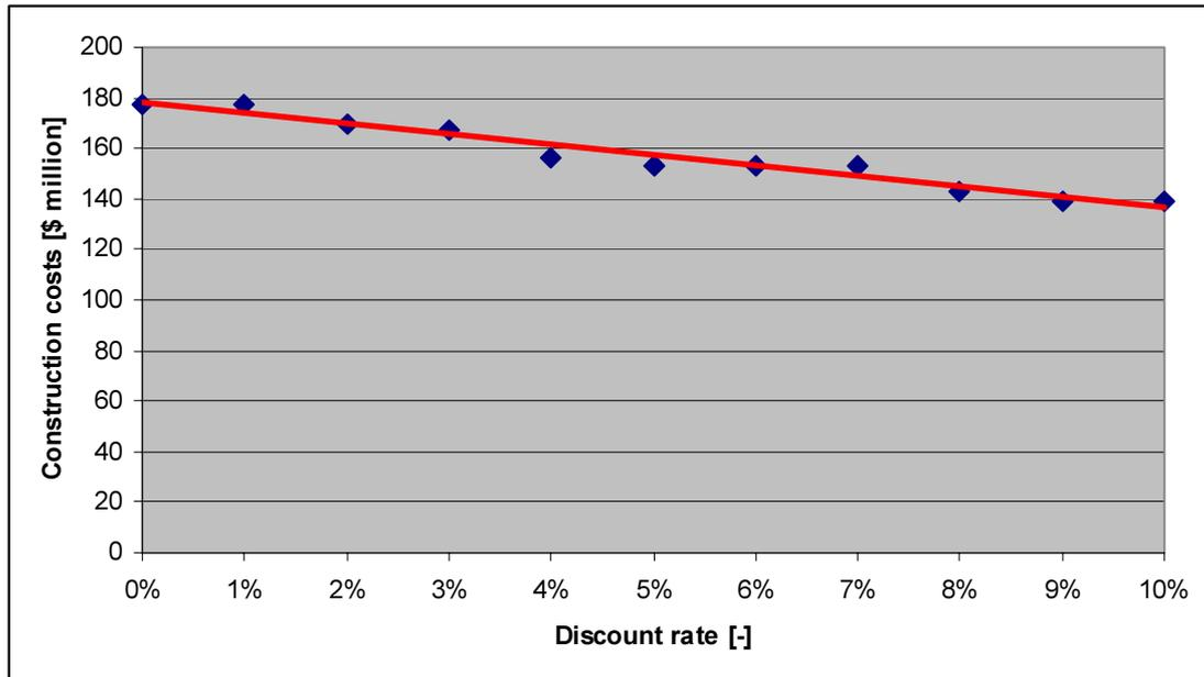
Figure 57 Influence discount rate on construction costs
