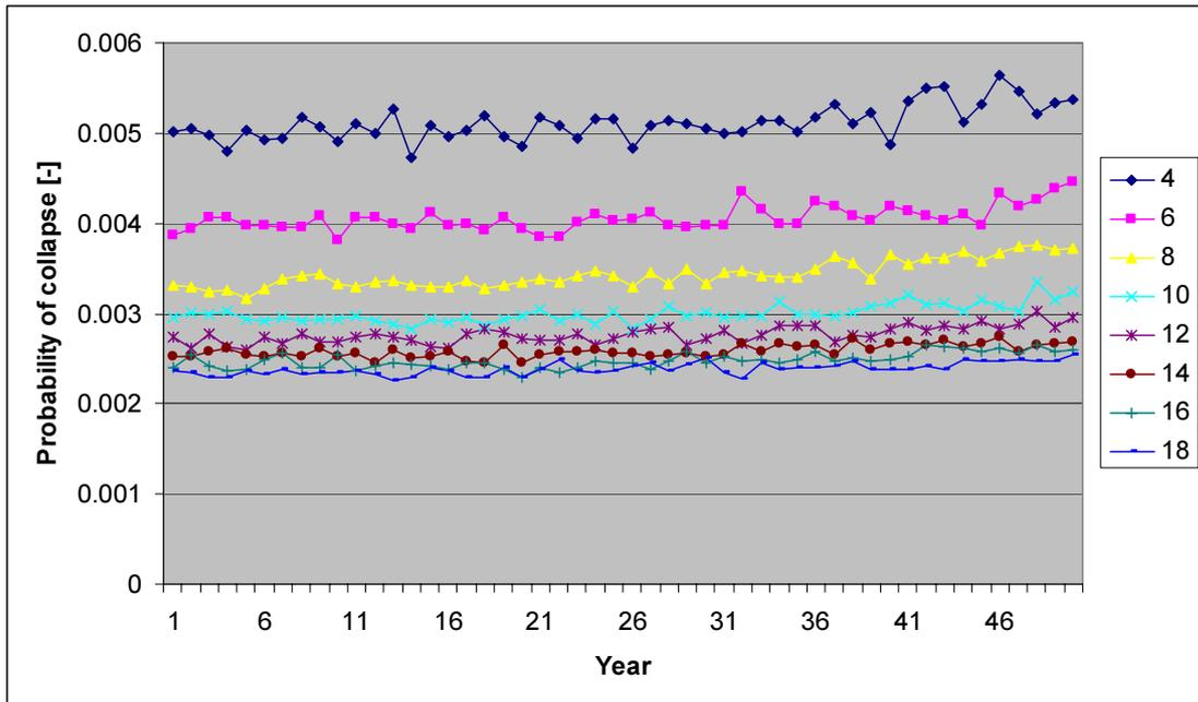
Figure 33 Probability of collapse due to hurricanes for all element volumes [ $\text{m}^3$ ]
