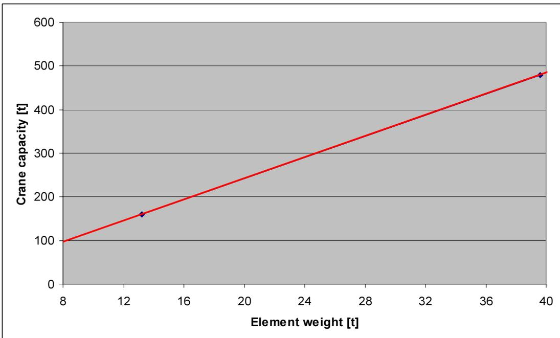
Figure 25 Crane capacity as a function of element weight
