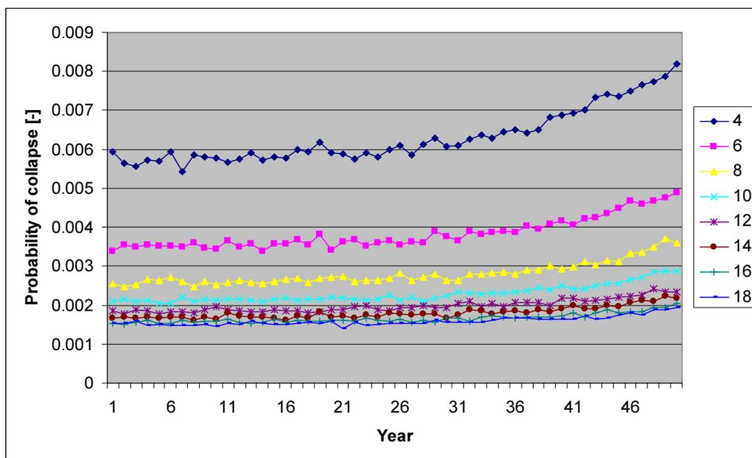
Figure 32 Probability of collapse due to Nortes for all element volumes [m<sup>3</sup>]
