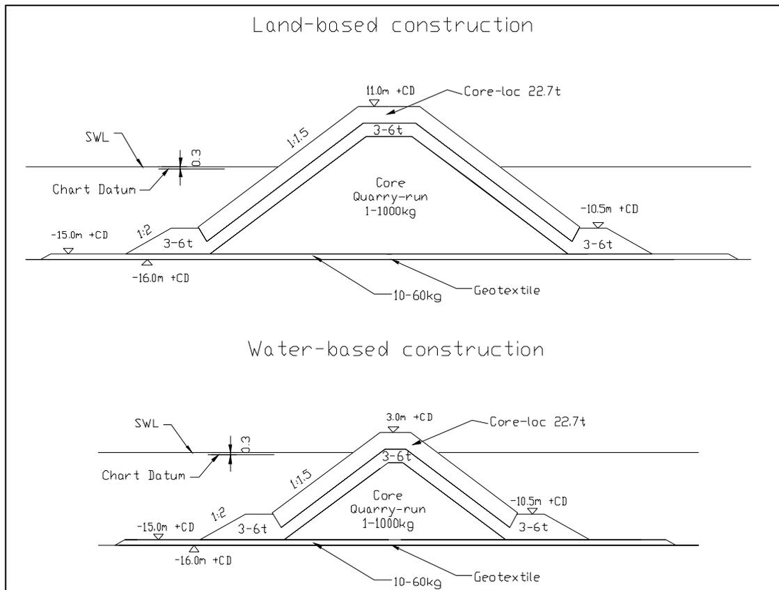
Figure 23 Breakwater cross-sections
