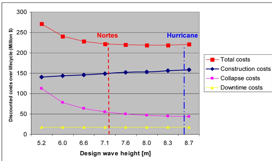
Figure 58 Discounted costs for the significant design wave height variation
