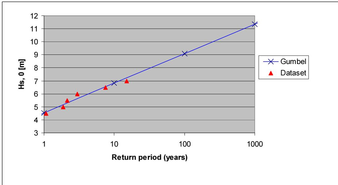
Figure 7 ULS significant wave height exceedence probability
