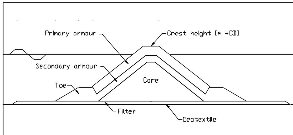
Figure 20 Breakwater components
