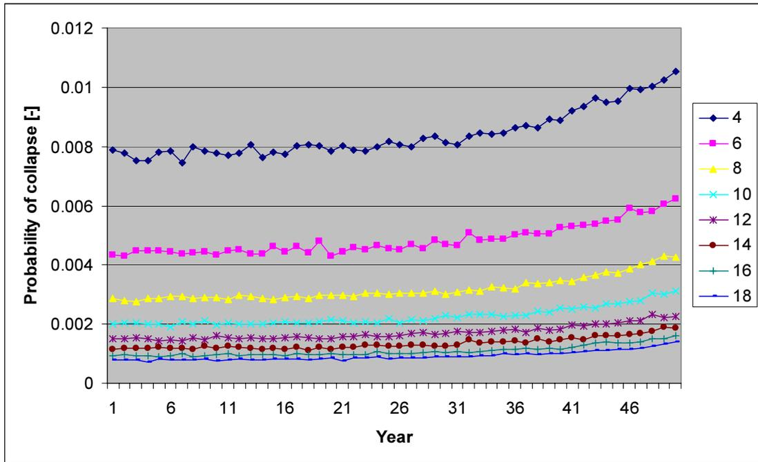
Figure 30 Probability of collapse due to Core-loc® armour failure for all element volumes [m<sup>3</sup>]
