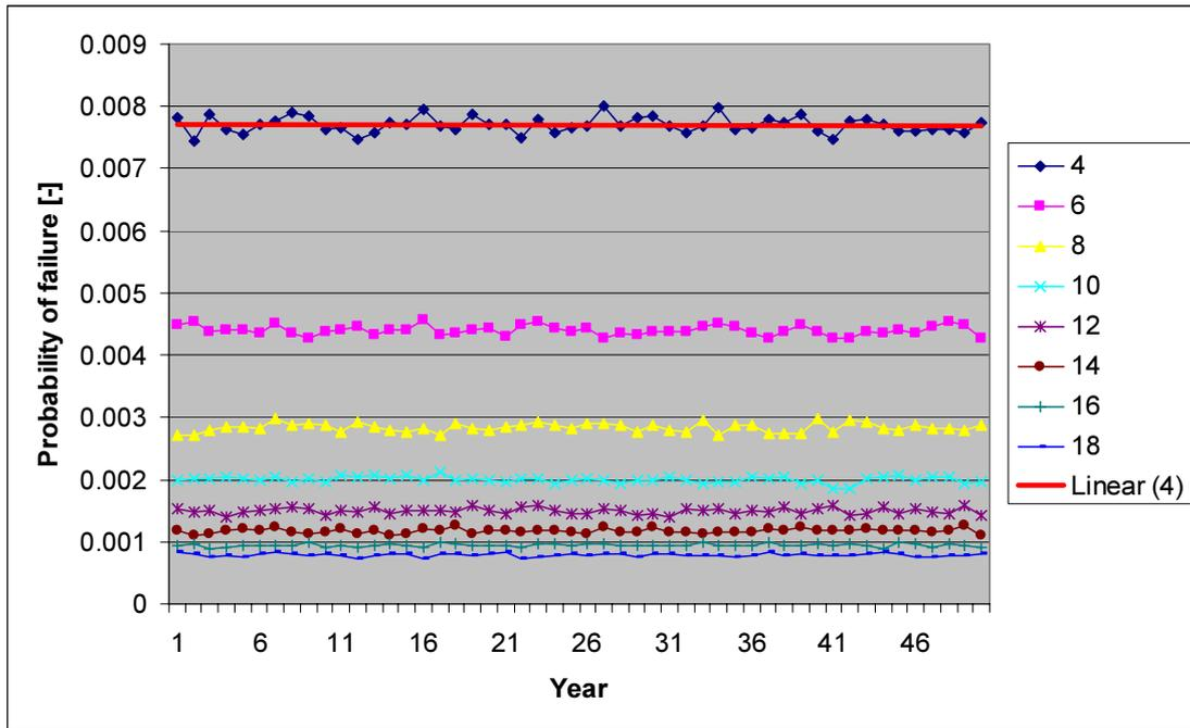
Figure 35 Probability of collapse for Core-loc® armour without deterioration of strength for all element volumes [m<sup>3</sup>]
