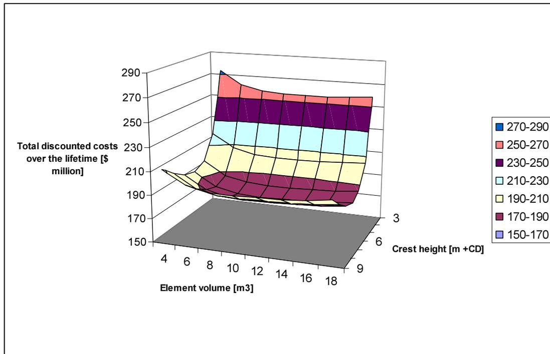
Figure 56 Total discounted costs with a discount rate of 10%
