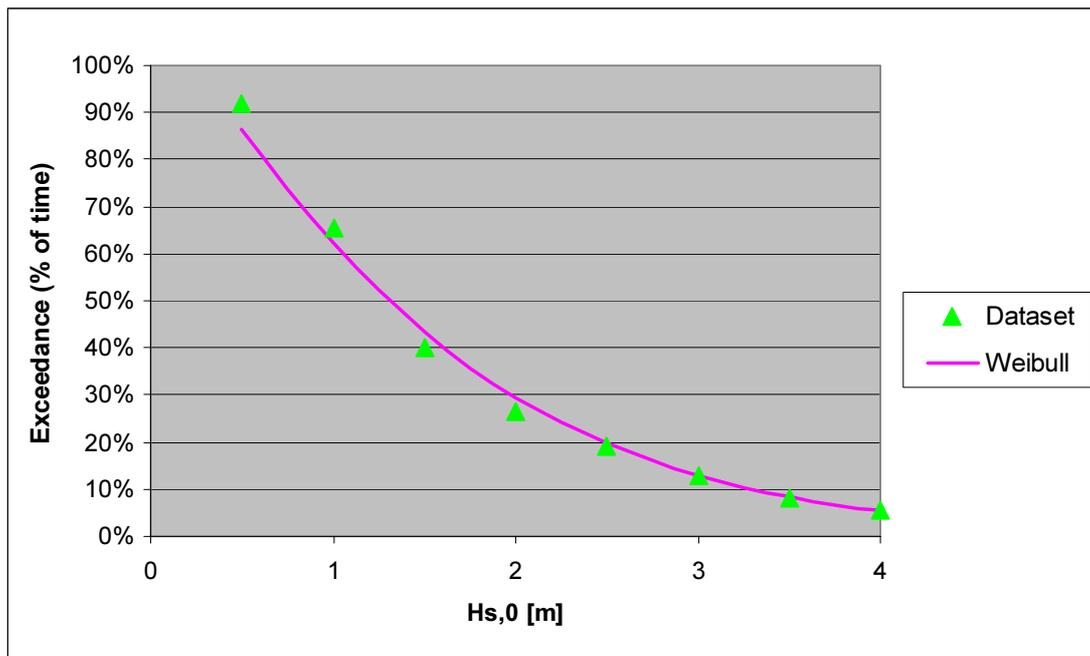
Figure 8 Significant wave height distribution in % of the time
