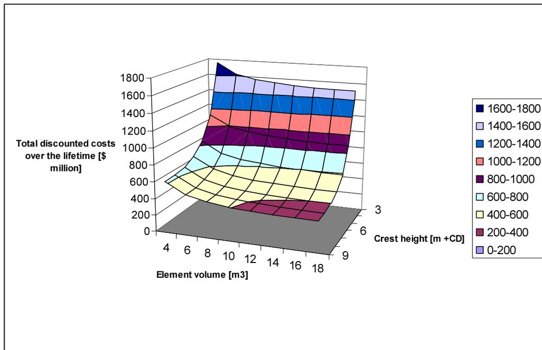
Figure 55 Total discounted costs with a discount rate of 0%
