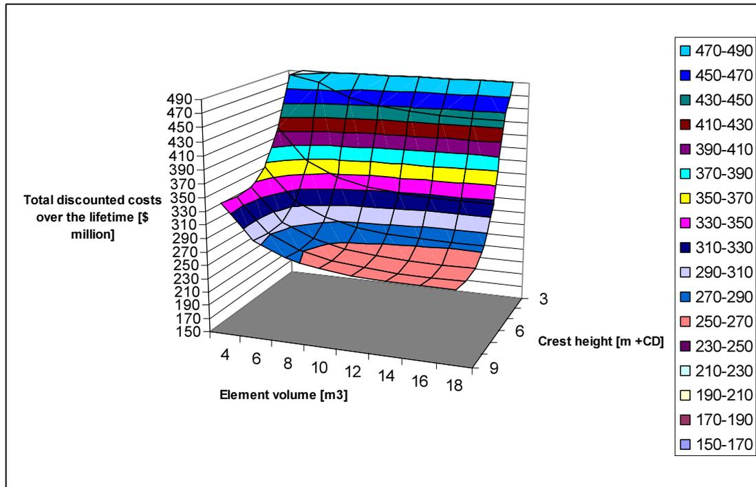
Figure 53 Total discounted costs over the lifetime with a 7% throughput growth rate [\$ million]
