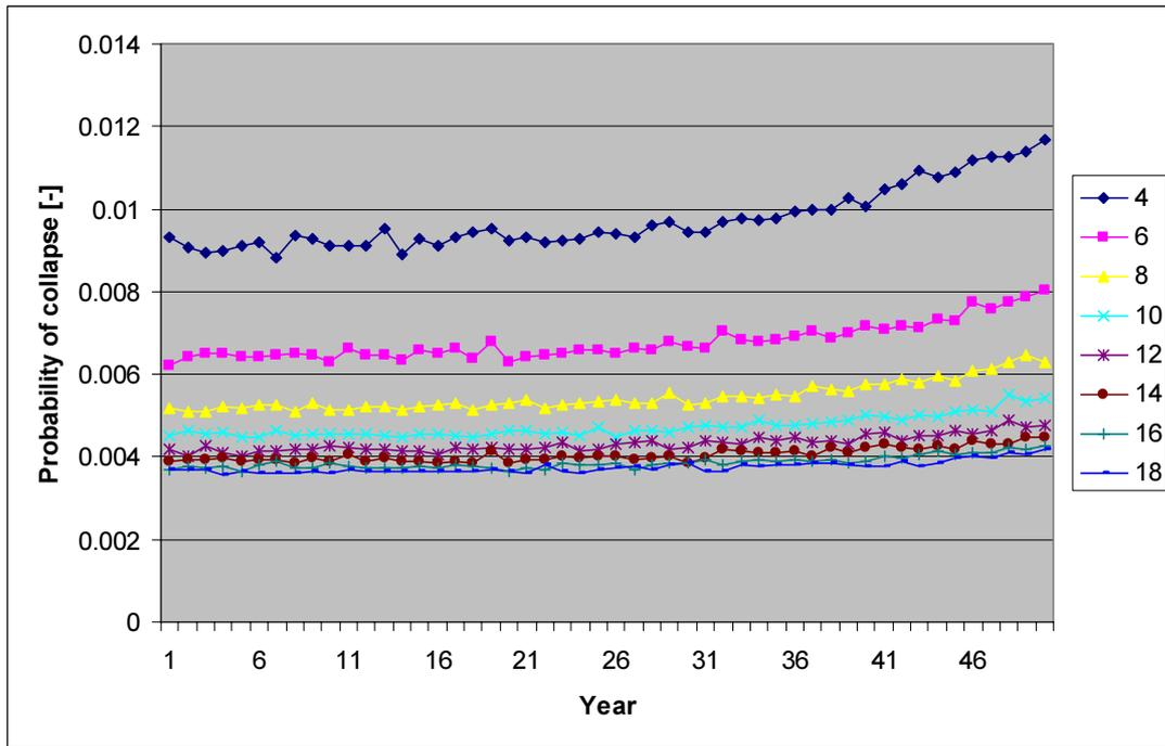
Figure 34 Probability of collapse for the breakwater for all element volumes [m<sup>3</sup>]
