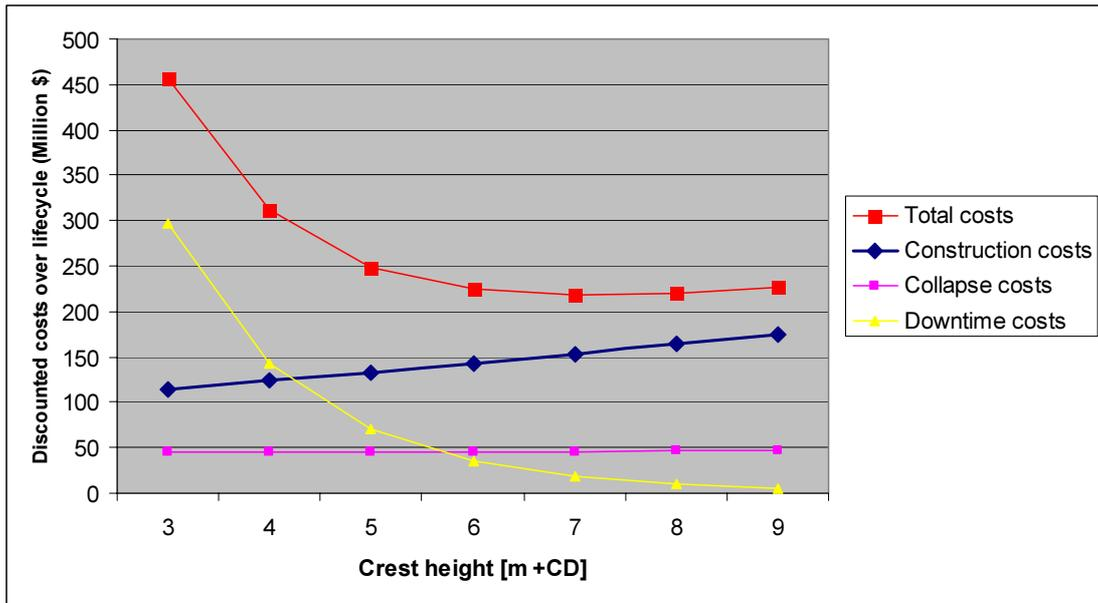
Figure 47 Costs for crest height variation for an element weight of  $14\text{m}^3$
