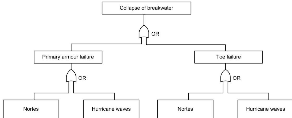
Figure 28 Fault tree for collapse of breakwater
