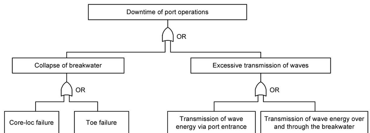
Figure 4 Fault-tree for a breakwater
