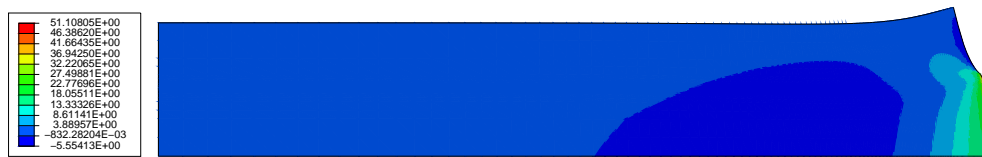
Figure 3.4: Distribution of interlaminar normal stress \sigma_z (MPa) for 876 elements
