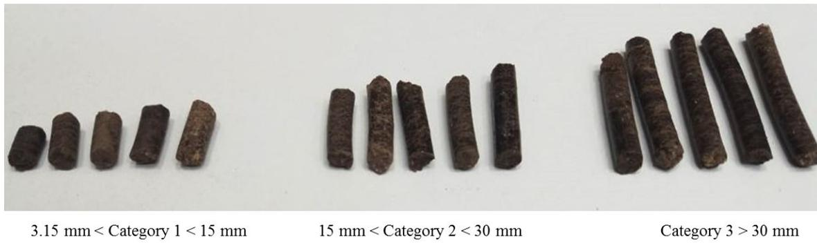
Figure 3.1: Samples of different categories of torrefied mixed wood pellets.
