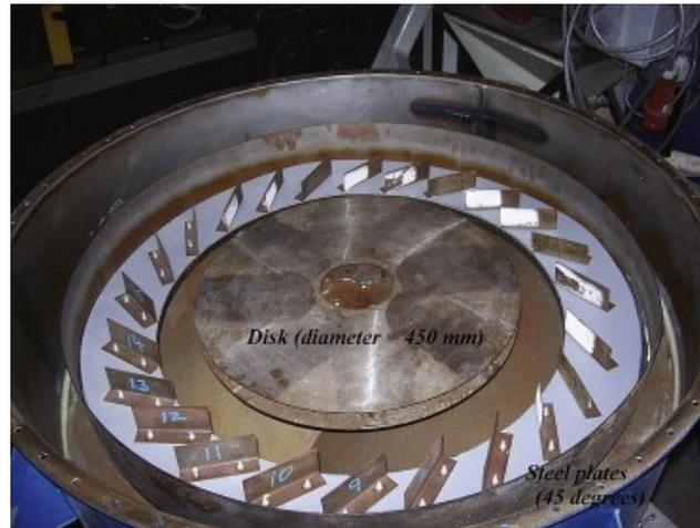
Figure 2.10: Rotary impact test apparatus of the University of Greenwich [78].
