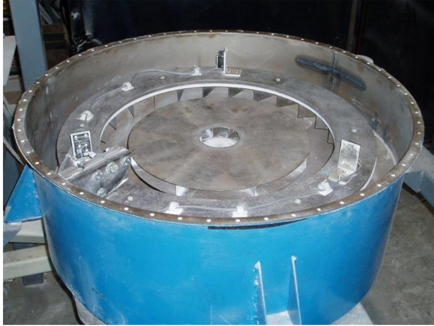
Figure 4.2: Rotary impact tester.
