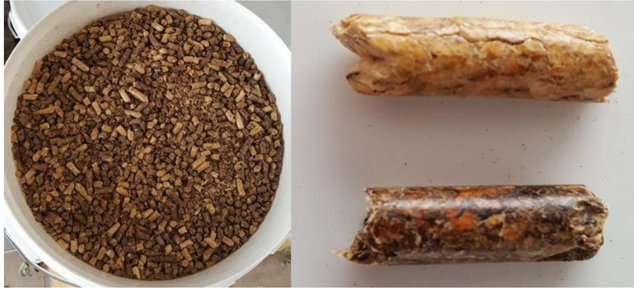
Figure 4.1: Wood pellets used in the experiments: a bucket of mixed pellets (left), the two different types of wood pellets in a close-up (right).
