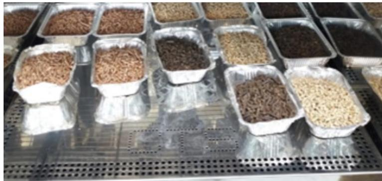
Figure 6.1: Pellets on aluminum trays in the climate chamber. This figure is an example showing the pellets on aluminum trays. The same trays were used for the other storage conditions.
