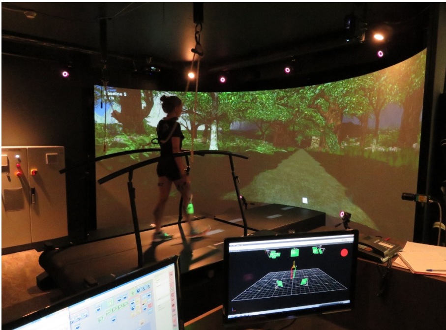
Figure 1) Motek C-Mill treadmill with virtual environment – Step targets were presented on the Motek C-Mill treadmill band for the left and right foot. Targets first appeared in the virtual environment, sequentially, they appeared on the treadmill band. Subjects walked with their head straight, looking at the virtual environment. This way, the walking task would resemble overground walking. When subjects stepped in a target, the target turned green and an auditory 'beep' was presented. When subjects missed a target, the target turned red. Ground reaction force plates were integrated in the treadmill band ( f_{GRF} = 100 \text{ Hz} ). The weight bearing mechanism and the handrails of the C-Mill were not used in our study.
