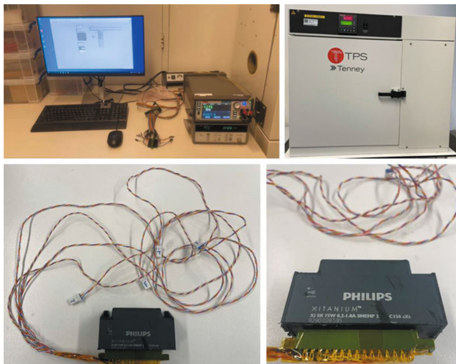
Fig. 13.9 Test equipment (top) and driver modules (bottom) used for PHM
