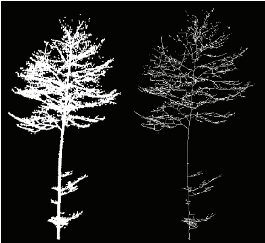
Figure 7.1: (left) point cloud of a tree with leaves and (right) the SkelTre skeleton corresponding to the point cloud on the left
