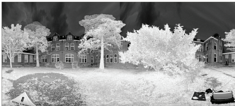
Figure 1.2: Intensity image of a panoramic laser scan
