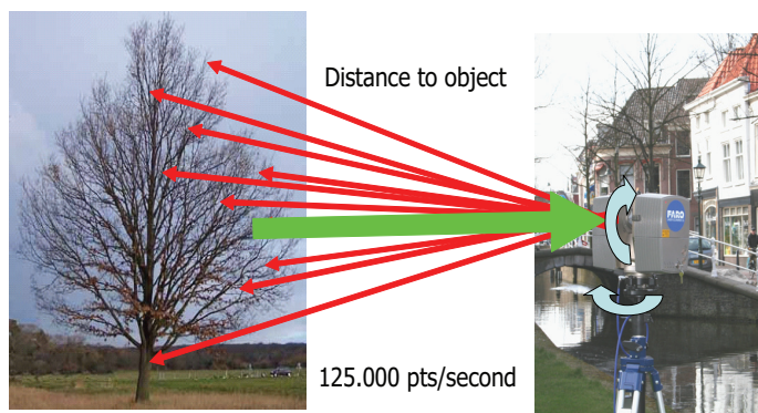
Figure 1.1: Simplified scanning principle of a terrestrial laser scanner
