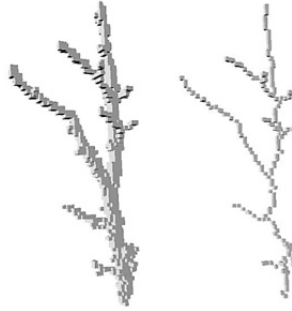
Figure 3.3: Skeleton extracted by morphological thinning with the algorithm of [Gorte and Pfeifer, 2004]. (Left) non-empty voxels (right) extracted skeleton
