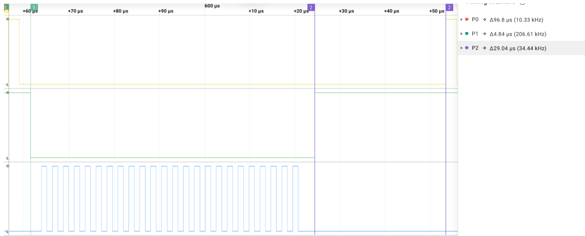
Figure 7.5: Logic analyser capture of the ADC conversion timing sequence
