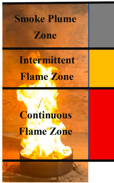
Fig. 14. The structure of the pool fire plume.
