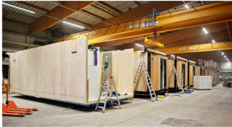
Figure 18 Assembly of Finch CLT modules (Finch buildings, 2020)
