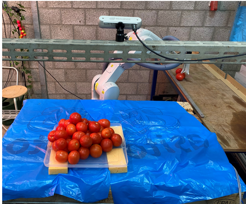
Figure 5.2: Overview of the setup, showing the camera placed above the tomatoes, and a storage table on the right, where the tomatoes will be deposited.
