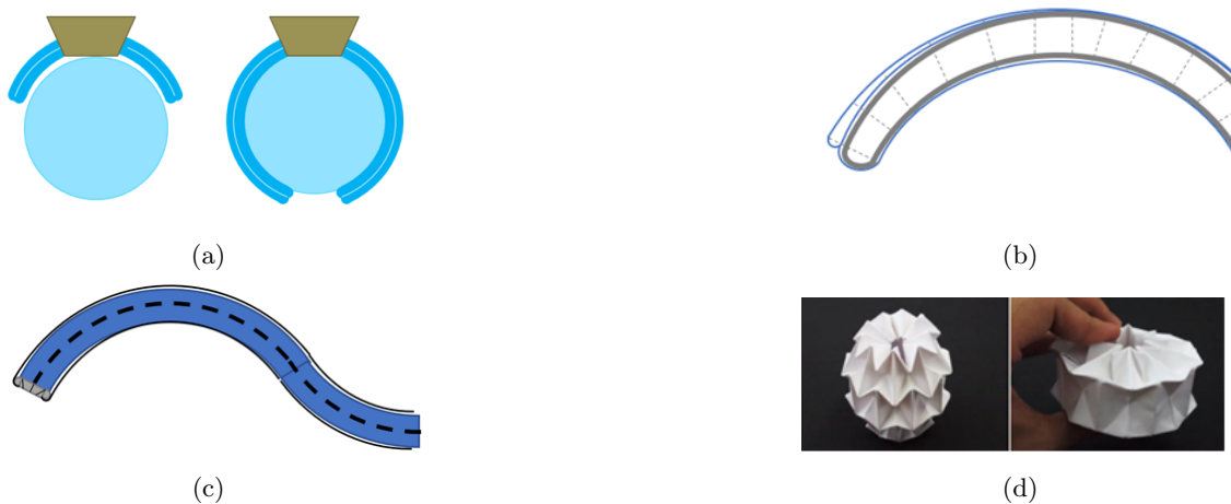
Figure 3.5: Different implementations for using an eversion mechanism with some sort of method for increasing bending stiffness. Figure (d) was adapted from [Lee et al., 2013].
