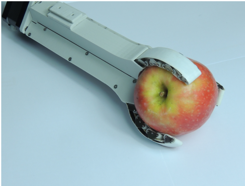
Figure 4.15: Prototype of the designed gripper, in its fully assembled and functional form, holding an apple.
