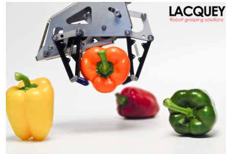
(b) Underactuated finger gripper designed by Lacquey. Retrieved from [Lacquey, nd].
